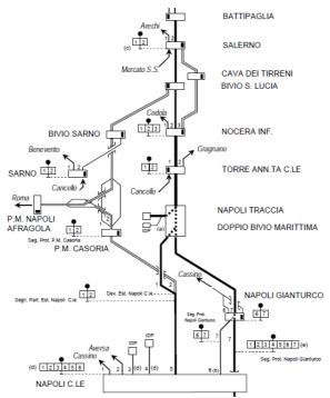
Figure 15: Schematic layout of the Napoli Centrale- Salerno line by RFI
