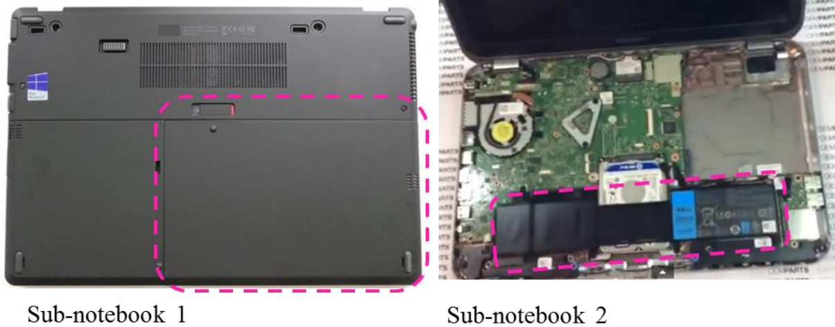
Figure 7. Location of the battery pack in two subnotebook computers: subnotebook 1 with external accessible battery pack, and subnotebook 2 with embedded battery pack accessible only after the base cover is unscrewed and the palm rest removed.
