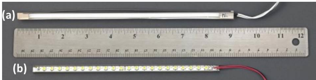
Figure 12. CCFL tube backlight units (a) are rapidly giving way to LED strings or rails (b) for LCD backlighting (Barney 2013).
