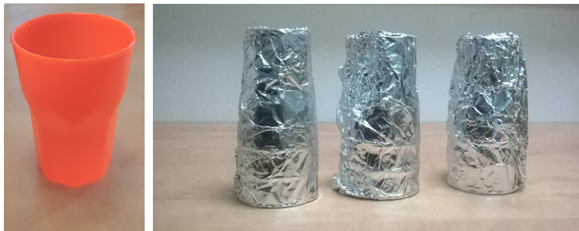
Figure 1. Polypropylene (PP) cups (left) as prepared for shipment (right)
