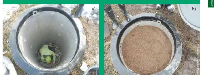
a) Lysimeter and b) soil column for an in situ pilot test at the UHEL lysimeter field station.
