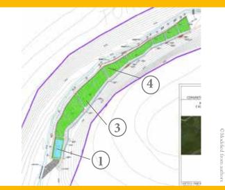
Final layout (3. anaerobic, 4. aerobic, 1. sedimentation)
