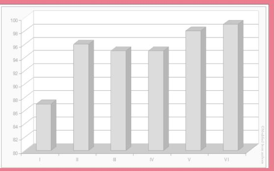
Average plant coverage (%) as response to the stabilization treatment at Piekary Site II recorded in 2012 (15 years after the treatment). Plots I-VI correspond to low B; high B; low B + low BL; high B + low BL; low B + high BL; high B + high BL, respectively (B-biosolids, BL-byproduct lime). No plants grown at untreated control area.
