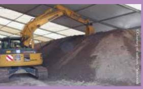
Dynamic aeration cycle using a bucket excavator
