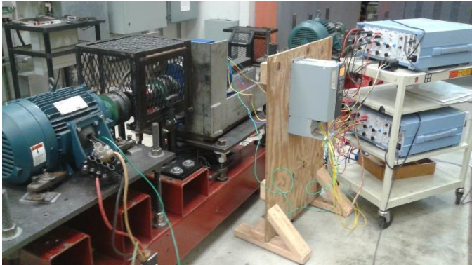
Fig 10: A 7.5hp motor-drive system under test
