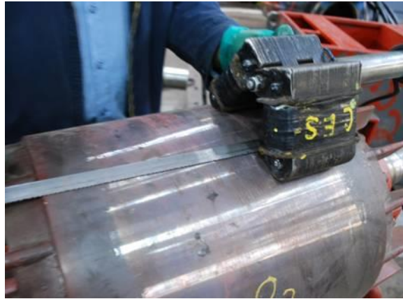
Figure 6: Growler test of a rotor.
