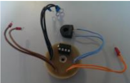
Figure 3: Sensor module to be mounted inside the pump
