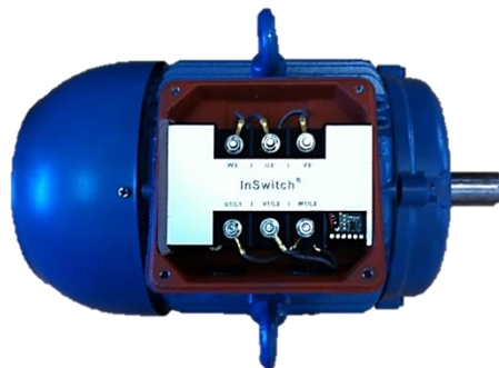
Fig. 2. InSwitch installed inside the terminal box of a 7.5-kW, 4-pole SCIM.
