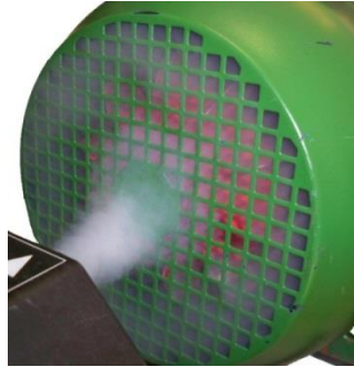
Fig. 10. Smoke test performed on the original ventilation system (centrifugal fan plus cover) of a 7.5-kW, 4-pole, 50-Hz, 3-phase, self-cooled, induction motor to observe the airflow behavior and visualize the recirculation inside the cover.
