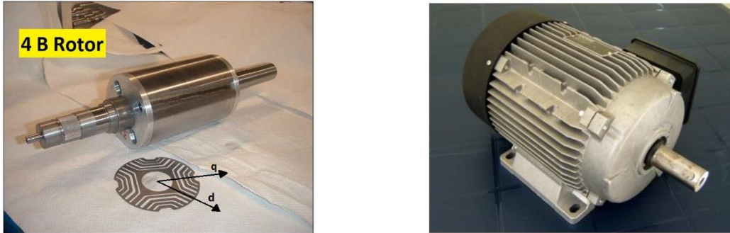
Figure 1: Optimized SRM: rotor core with denoted the direct (d) and quadrature (q) axes (left) and its assembly in the case of a standard 3kW induction motor (right).
