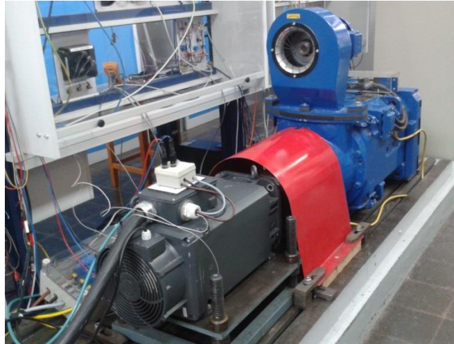
Fig. 3: Test bench with Machine 4 (on left-hand side) and a DC railway motor as load
