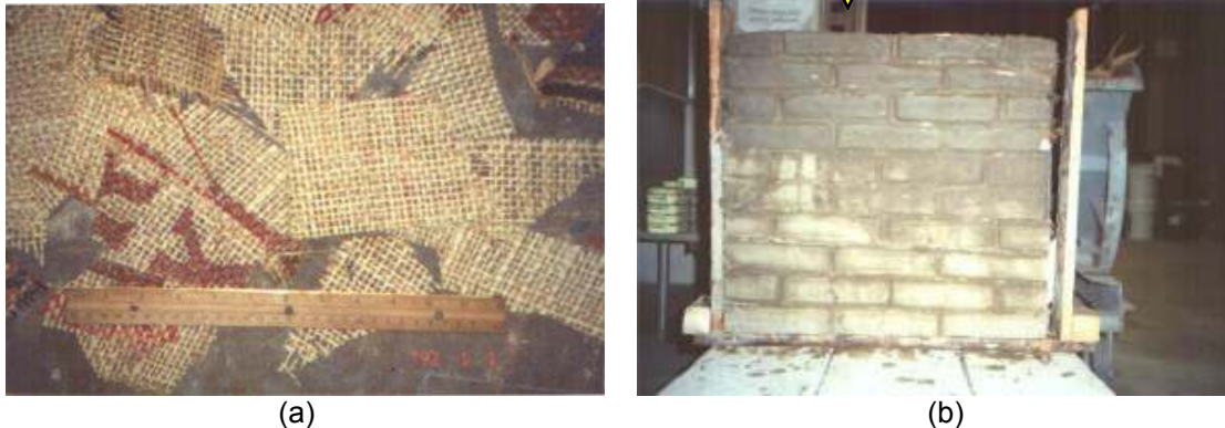
Fig. 4-18 (a) Burlap pieces cut from coffee bags; (b) Control specimen in the process of drying. (source: http://www.engineering4theworld.org/adobe.html )
