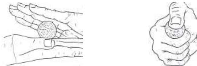
Fig. 3-13 Dry strength test of soil, as per IAEE, 1986.
