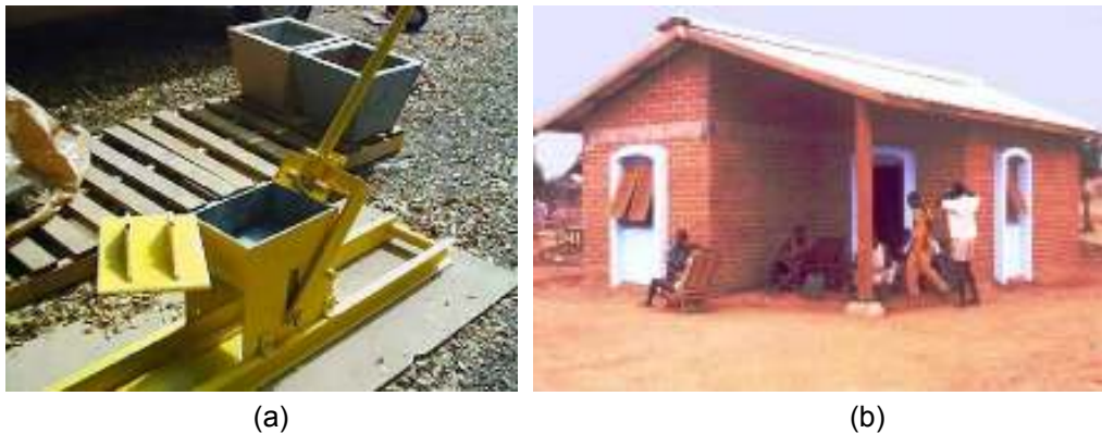
Fig. 3-31 (a) A “Cinva ram” press; (b) This house was built using compressed earth bricks in Ivory coast, within 10 days, by trainees, who were part of a local development program. [sources: (a) http://www.northcoast.com/~tms/adobe.html ; (b) http://www.earth-auroville.com ]
