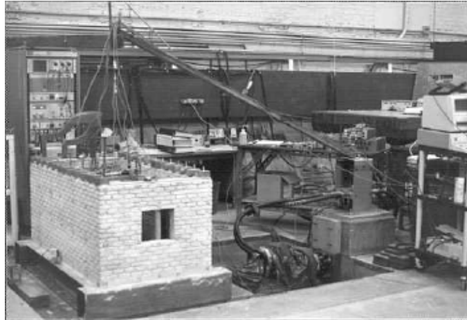
Fig. 4-17 Specimen mounted on the seismic table.
