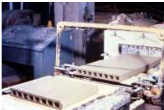
Fig. 3-32 Extruded earth profiles production line. (source: unknown)
