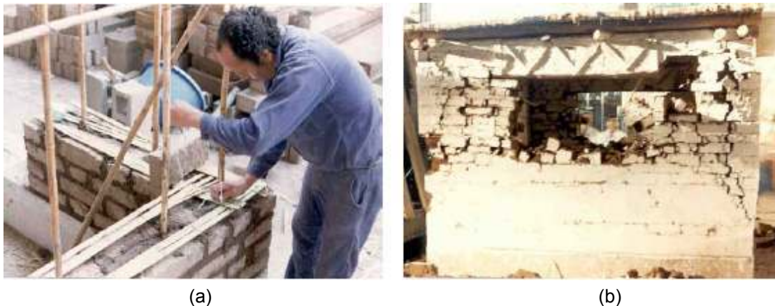
Fig. 4-11 (a) Cane reinforcement; (b) Reinforced module after a seismic test.
