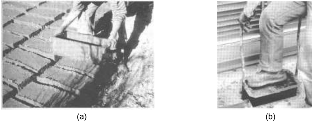
Fig. 3-36 (a) Arrayed adobe bricks, left to dry in the sun (Ecuador); (b) Releasing adobe brick off the (metal) mould. (source: Minke, 2000a)
