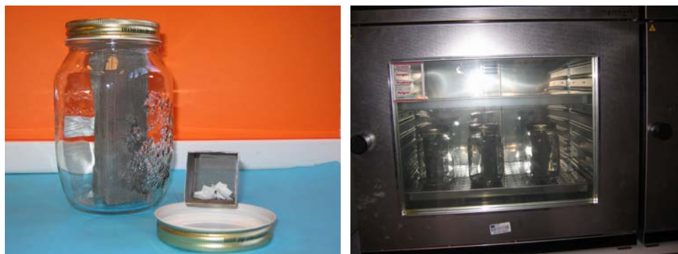
Picture 2: a) Sample vessel and b) oven for method EN ISO 14184-2.
