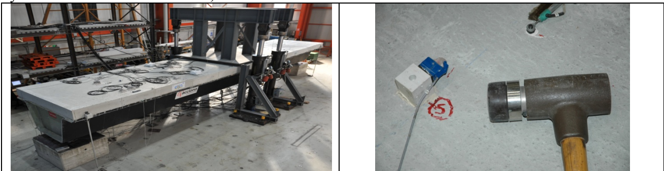
Figure 1: General view of the structure on left and input (Hammer) and output (Accelerometer) transducers used for modal testing
