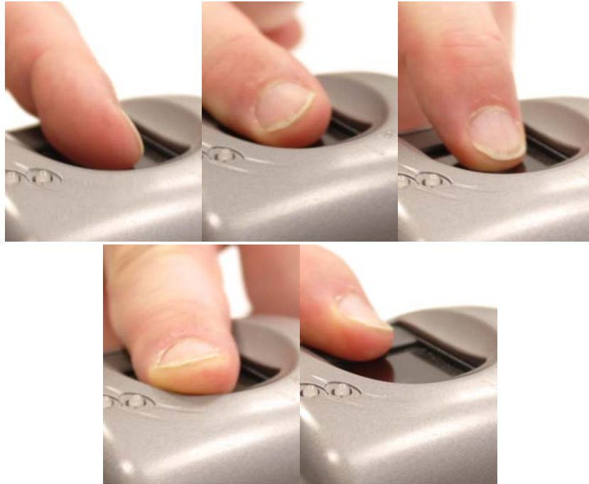
Figure 4: Wrong positioning of the finger on a scanning device (too far turned to left side; too far to right side; too steep; too much advanced; too less advanced)
