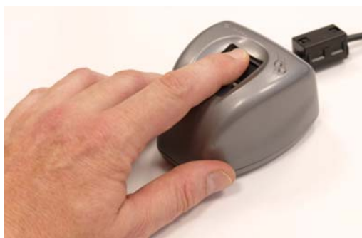
Figure 3: Acquisition of a fingerprint from an index finger by a commercial scanning device
