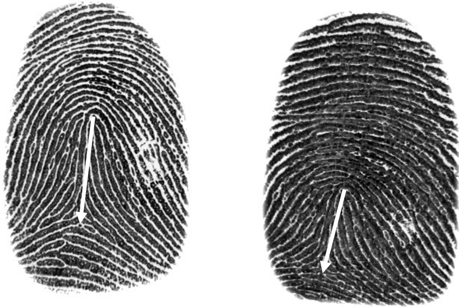
Figure 29: "Normal" and strongly distorted fingerprint image of the same finger The white arrows denote the distance between the same landmarks in both prints. 23
