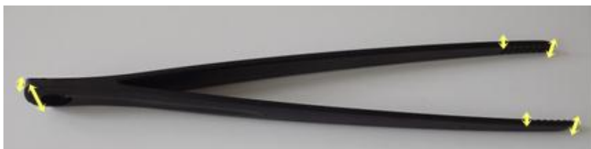
Figure 14 Dimensions measured for homogeneity testing (Sample E)
