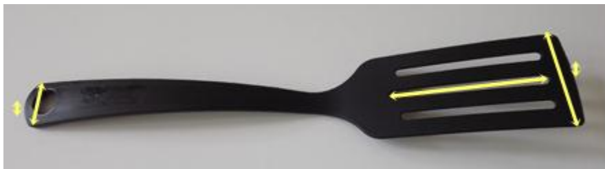
Figure 10 Dimensions measured for homogeneity testing (Sample A)
