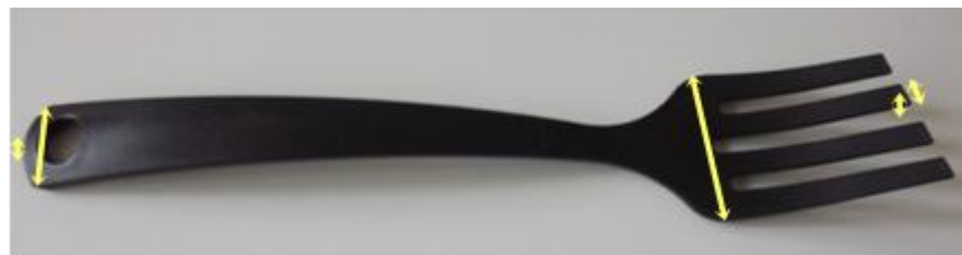
Figure 11 Dimensions measured for homogeneity testing (Sample B)
