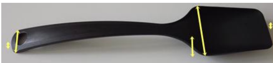
Figure 13 Dimensions measured for homogeneity testing (Sample D)
