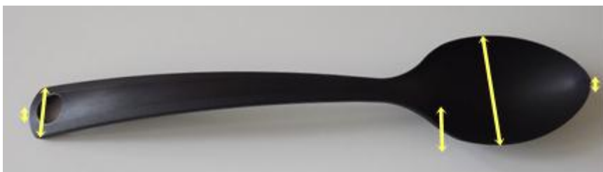
Figure 12 Dimensions measured for homogeneity testing (Sample C)
