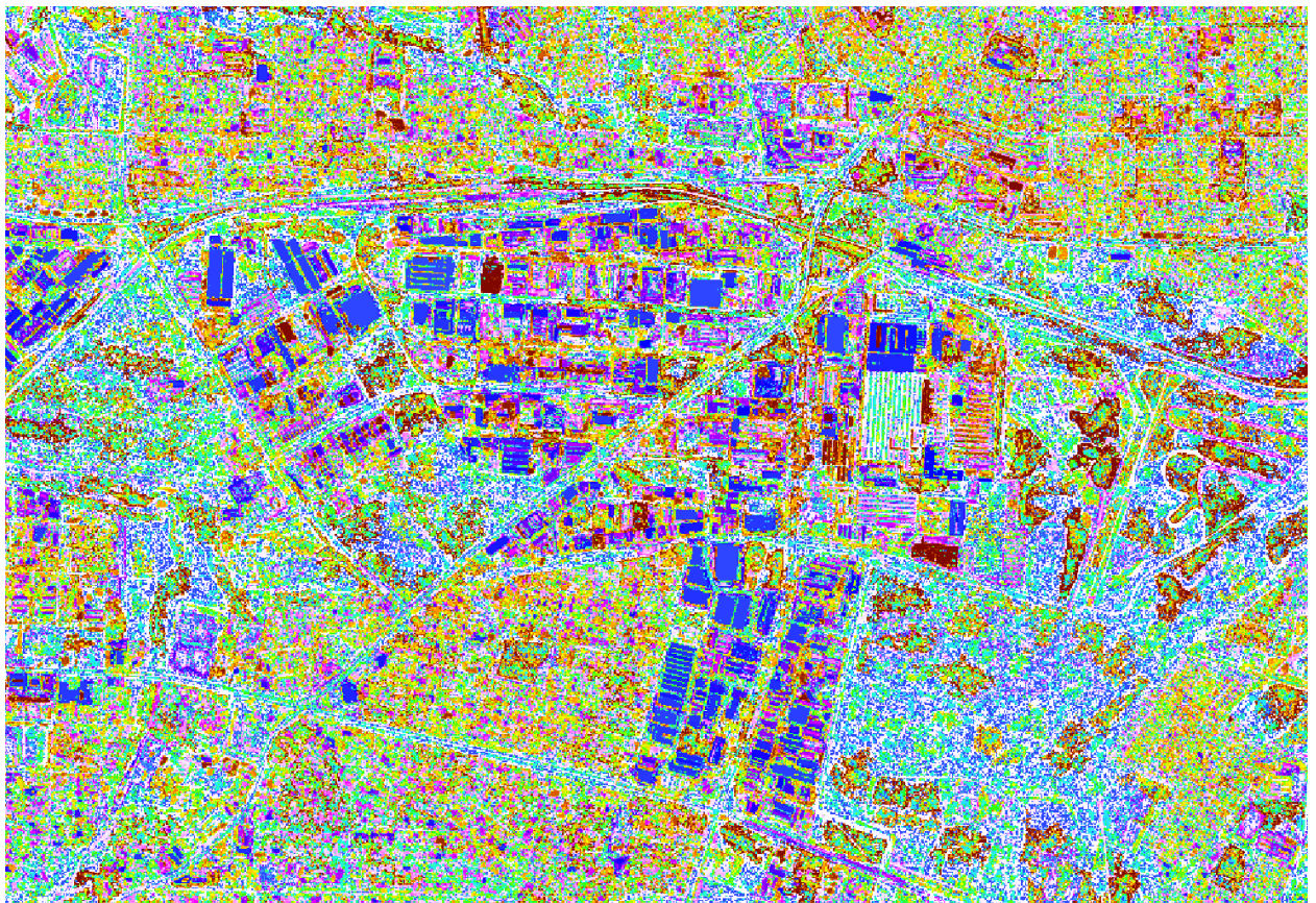
Figure 8. Exemplary output of the radiometric feature extraction. The colours mark similar features.
