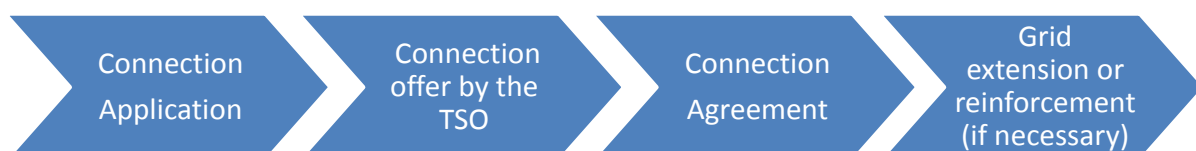
Figure 18: Grid connection procedure for offshore wind farms in the Netherlands.
