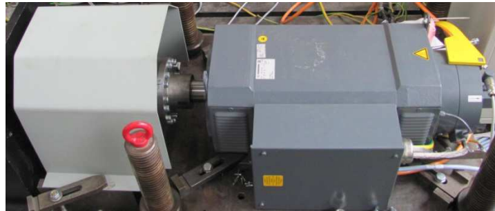
Fig. 8: Test bench with Machine 3 (on right-hand side) and Machine 2 as load
