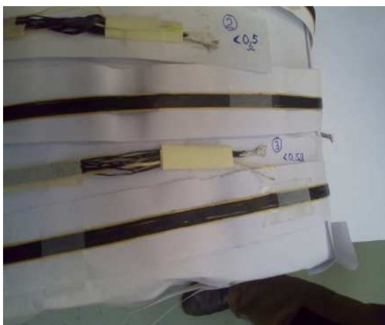
Figure 1: Ten parallel 26 AWG conductors (black ones) with aramid (Twaron) yellow yarns at the edges glued on aramid paper tape strips.
