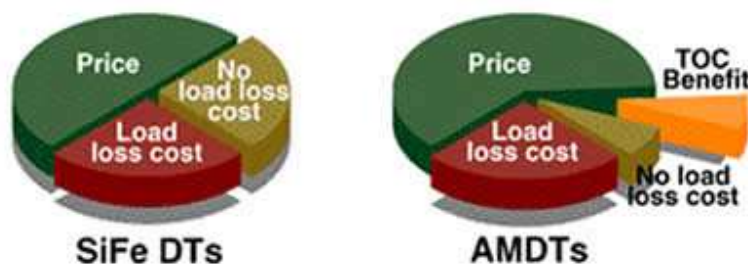
Figure 2: Cost and benefits of amorphous metal transformers (courtesy of Hitachi Metals [2])
