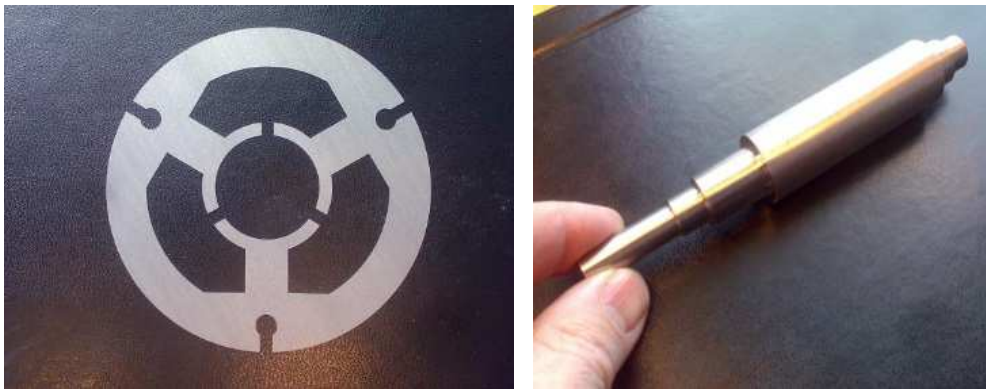
Figure 3: Stator lamination sheet on the left and the assembled PM rotor on the right.
