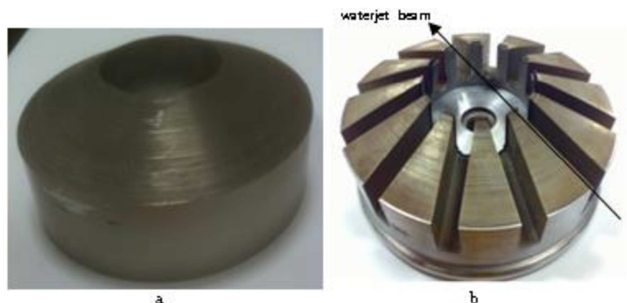
Figure 6: Water jet cutting of wrapped amorphous core [8]
