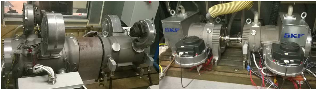
Figure 6 : Back to back test bench (left side: 90 kW range, right side: 150 kW range)
