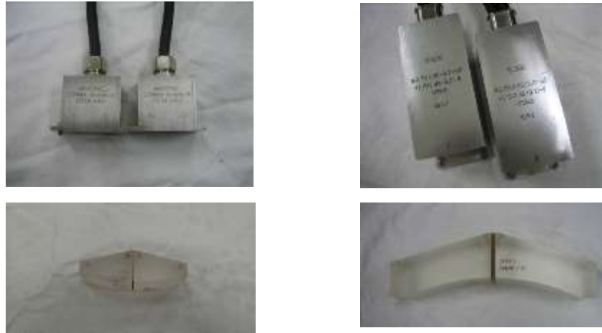
(a) 8x4 matrix probes and wedge
