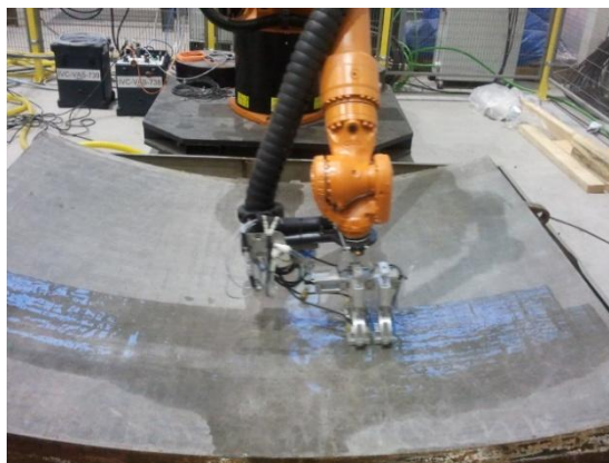
Figure 6. KUKA robot performing a scan on a wall mock-up
