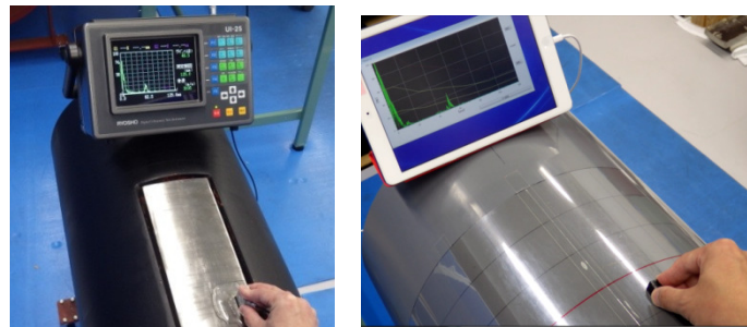
(a) UT work with specimen (b) UT work using virtual UT system
