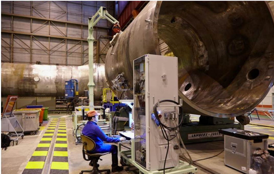
Figure 6: Dedicated automated UT system during commissioning in factory
