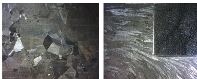
Figure 11. Macrographic representations of austenitic sample (left part) and DMW components (right part)
