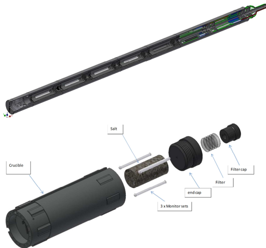
Figure 14: Representations of the SALIENT-01 sample holder containing 4 salt-filled and 1 empty graphite crucible (top), and of one graphite crucible (bottom).
