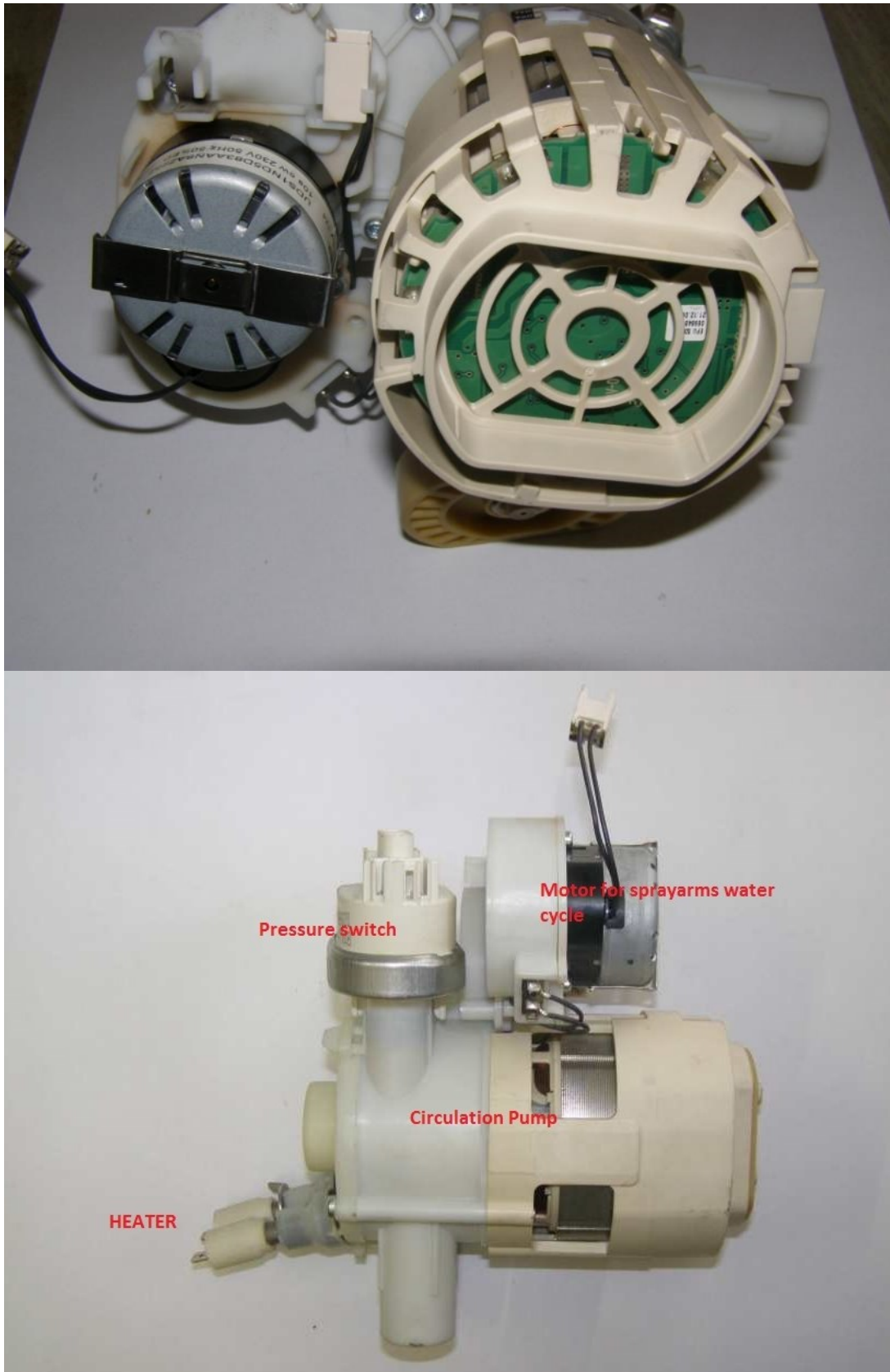
Figure 3.42. Circulation pump with electronic board — in case of failure, only the heater and the pressure switch can be replaced separately; the repair of other parts requires the replacement of the whole unit.
