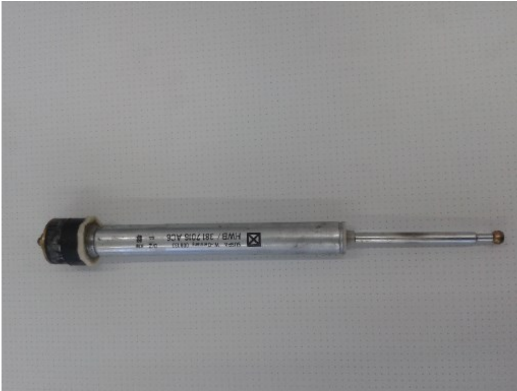
Figure 3.26. Shock absorbers (made of stainless steel) categorised as high-quality by the repair operator. By using four shock absorbers of this type, shocks are properly prevented and bearings are preserved.
