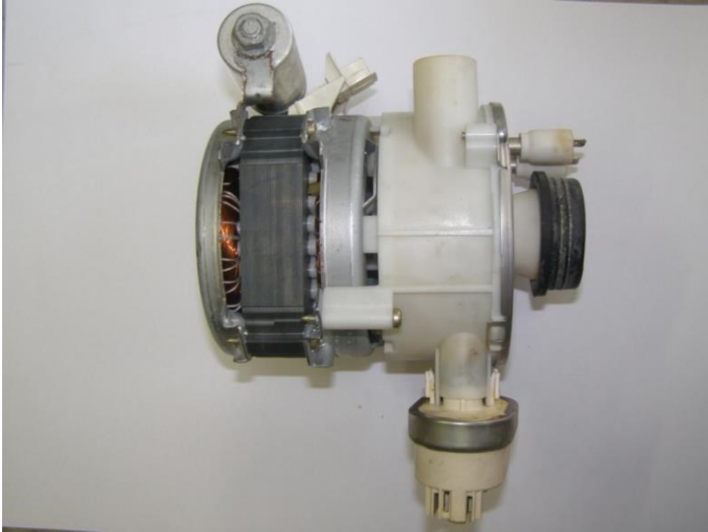
Figure 3.43. Circulation pump without electronic board — seals, pump, heater and motor are separable and their replacement does not require the whole unit to be replaced.
