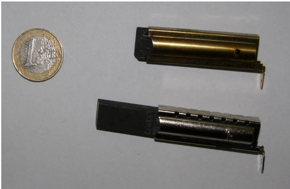
Figure 3.23. Worn-out carbon brushes (top) — as brushes wear out, they need to be accessible for maintenance or replacement with new carbon brushes (bottom)
