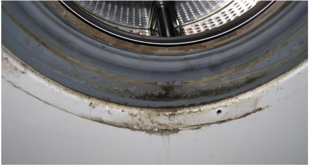
Figure 3.22. Worn-out door seal
