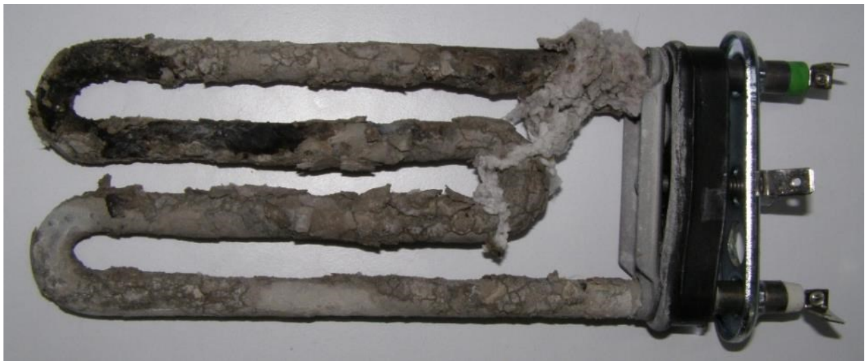
Figure 3.21. Contaminated and calcified heater
