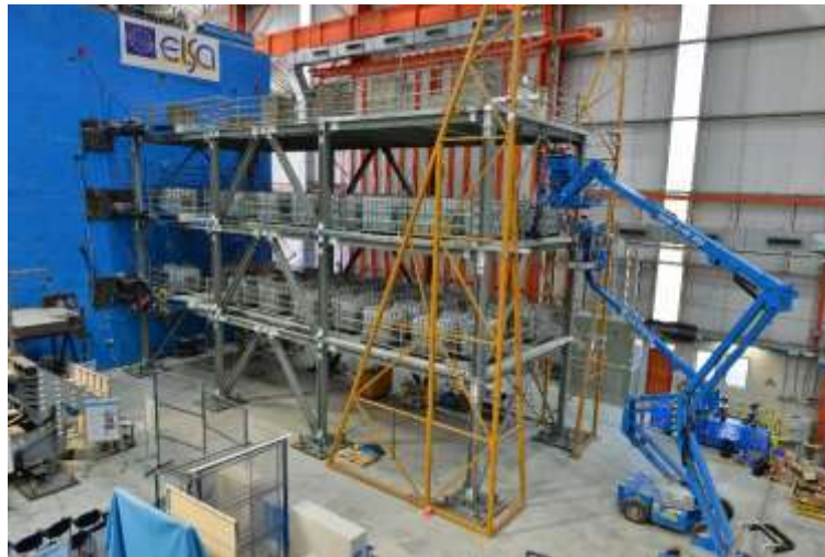
Fig. 2.1 View of the east platform of the ELSA reaction wall – strong floor facility
