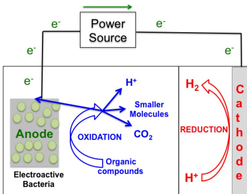
**Figure 3.** Working principle of a Microbial Electrolysis Cell (Courtesy of C. Santoro)
