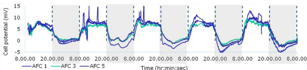
**Figure 5.** Voltage generated by three photo-MFCs over time (Courtesy of M. Di Lorenzo)
