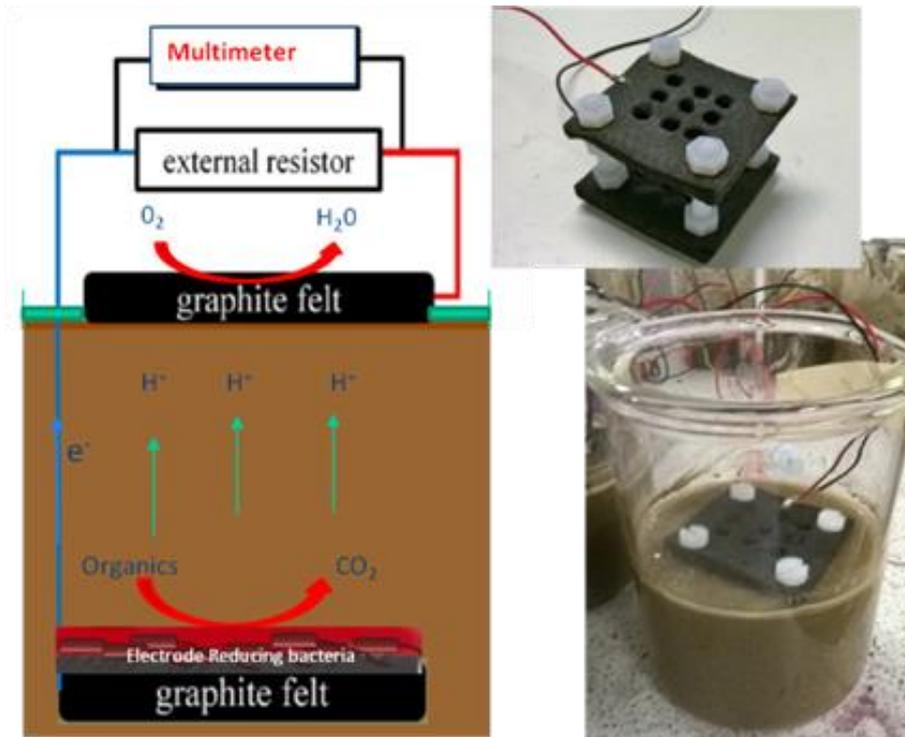
**Figure 4.** Scheme and photograph of a sediment MFC (Courtesy of M. Di Lorenzo)
