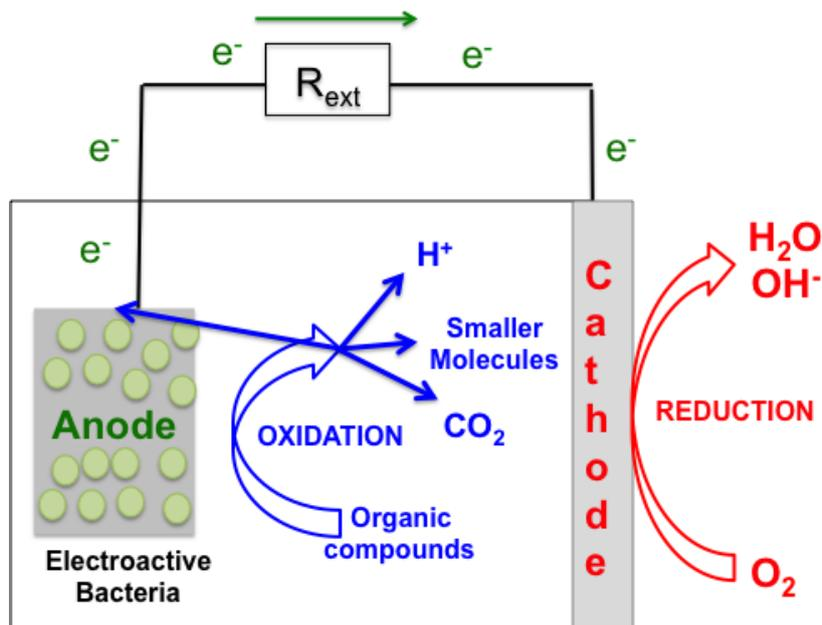
**Figure 2.** Working principle of a Microbial Fuel Cell (Courtesy of C. Santoro)
