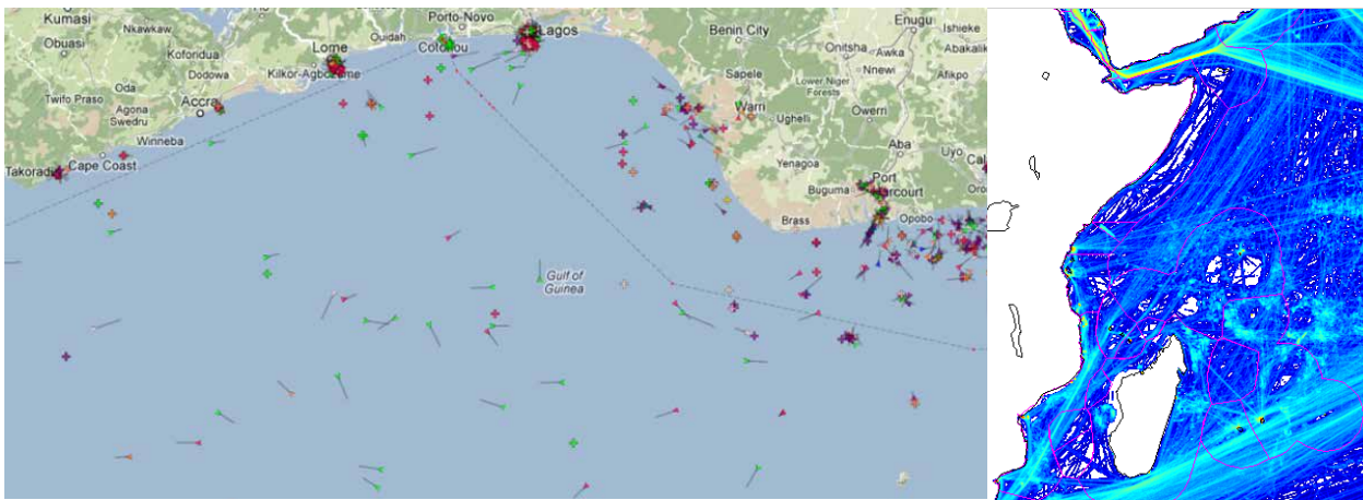
FIGURE 92: (left): maritime situational picture in the Gulf of Guinea showing the positions, types (by colour) and movements of ships at a particular moment in time. (right): ship-density map based on one month of data (January 2015) from the Western Indian Ocean, showing the main traffic routes (light blue and yellow line bundles) and fishing activity (light blue cloudy areas) (Source: PMAR project, JRC)
