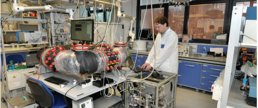
Validation of sensors to measure atmospheric particulate matter at the JRC-European Reference Laboratory for Air Pollution (ERLAP).
