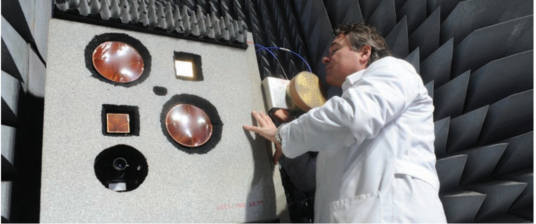
Fixing a circularly polarized antenna, designed for GNSS / Galileo applications, at the JRC-European Microwave Signature Laboratory.
