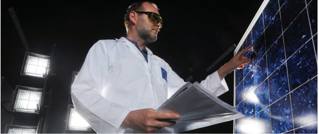
Class AAA solar simulator at the JRC-European Solar Test Installation (ESTI), devoted to the development of standards for electrical performance of photovoltaic products.
