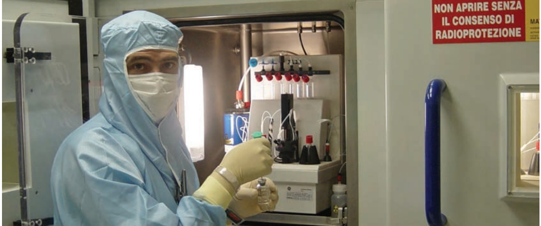
Preparing the automatic system for highly radioactive drug dispensing in the JRC radio-pharmaceutical laboratory.
