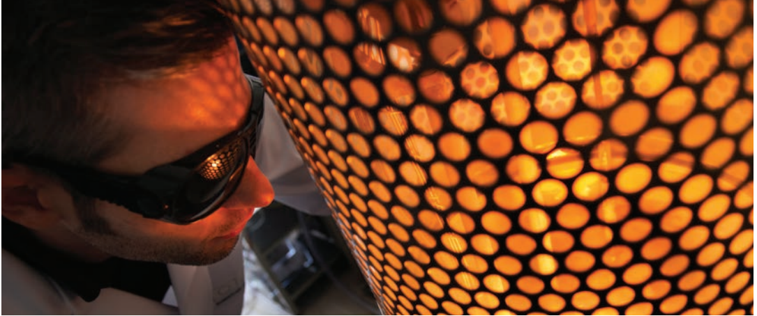
This lithium fluoride evaporator, for physical vapour deposition, is intended to improve nuclear safety and security. 2013.
