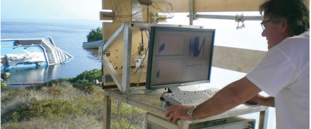
JRC researchers were monitoring the Costa Concordia shipwreck, thanks to the radar MELISSA (MIMO Enhanced Linear Short SAR), for more than two years.
