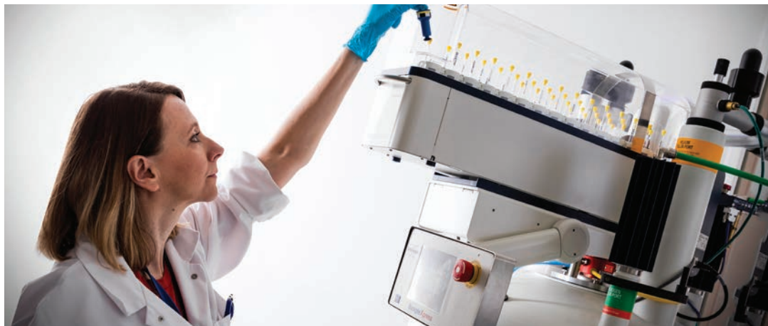
Testing wine samples in a nuclear magnetic resonance machine, at a JRC lab.
