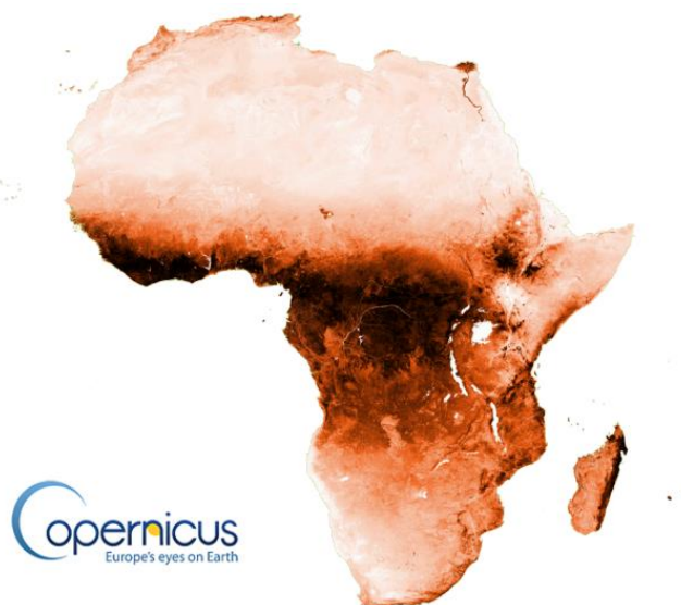
Figure 3: False color composite showing the biomass density, derived from Proba-V 100 m . The darker is more biomass. This was calculated on the Proba-V MEP in the frame of the Copernicus Global Land Service lot-1.
