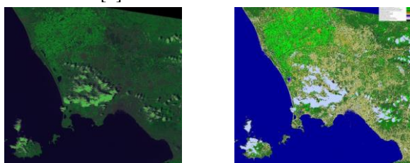
Left, Fig. 8(a). 4-band (B, G, R, NIR) ALOS AVNIR-2 image of Campania, Italy, radiometrically calibrated into TOARF values. Depicted in false colors (R = Visible Red, G = NIR, B = Visible Blue), 10 m resolution. No histogram stretching for visualization purposes. Right, Fig. 8(b). ESA EO Level 2 SCM classification map. Map legend shown in Fig. 4.
