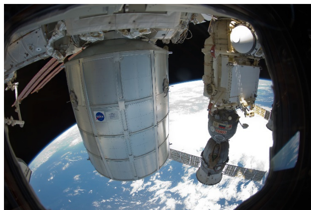
Figure 1: PMM docked to the Nadir port of ISS Node 1 during the STS-133 mission.
