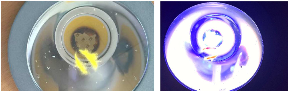
Figure 2: LED modules with remote-phosphor layer damaged. The blue LED chips are directly visible (Photo credits A. Barroso, LAPLACE Lab. 2016)
