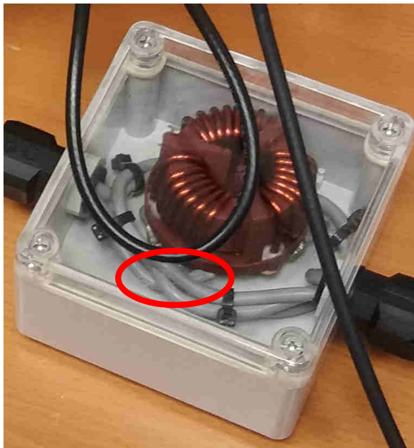
Figure 9: Unwanted cross coupling can be caused between the input and output cables seen inside the red circle
