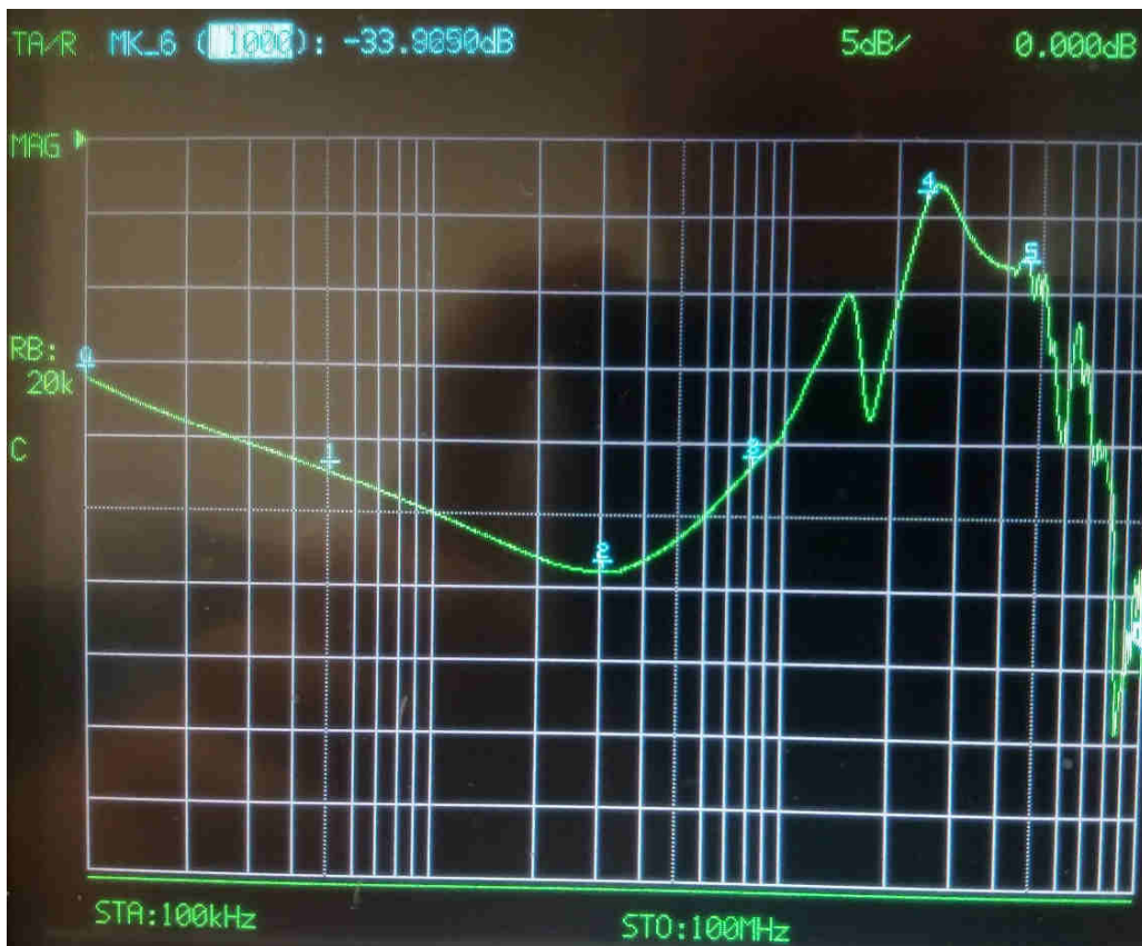
Figure 8: Common mode (rejection) response of the 3-line filter, measured at JRC
