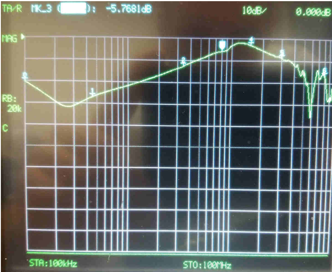
Figure 6: Measured common mode (rejection) response of FUSS-EMV filter with ground enclosure 'floating'
