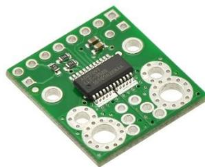
Figure 15. +- 75 Amps current meter
