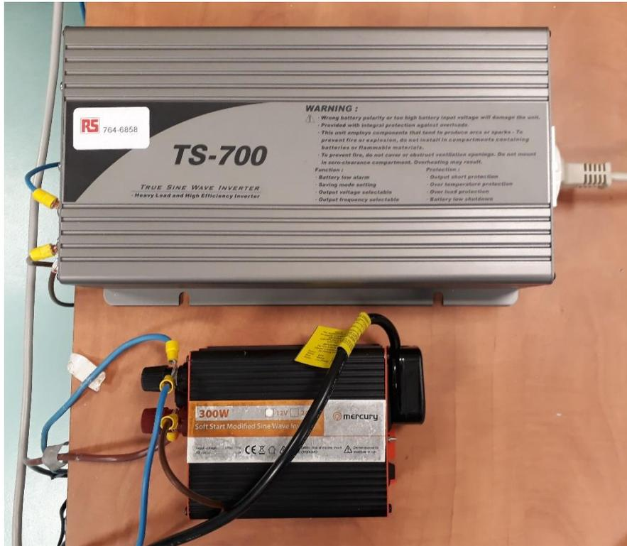
Figure 12. Off grid inverters
