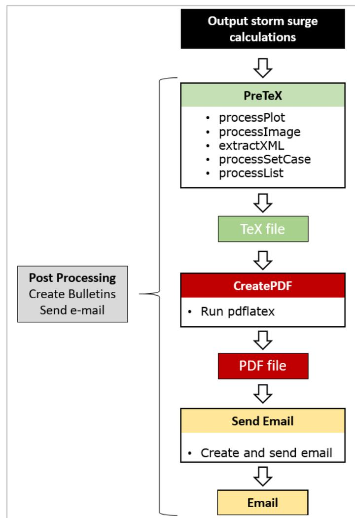
**Figure 6** - Procedures for the SSCS bulletins
