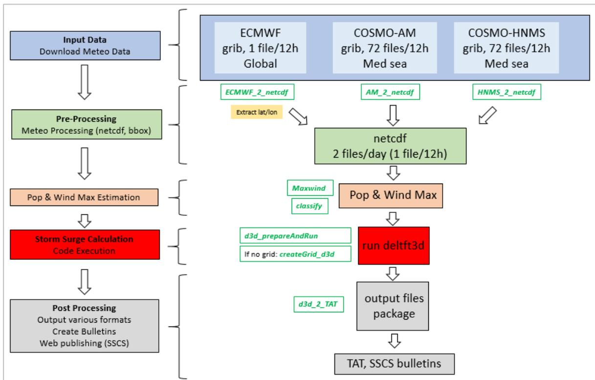
**Figure 4** – SSCS-Delft3D Procedure.
