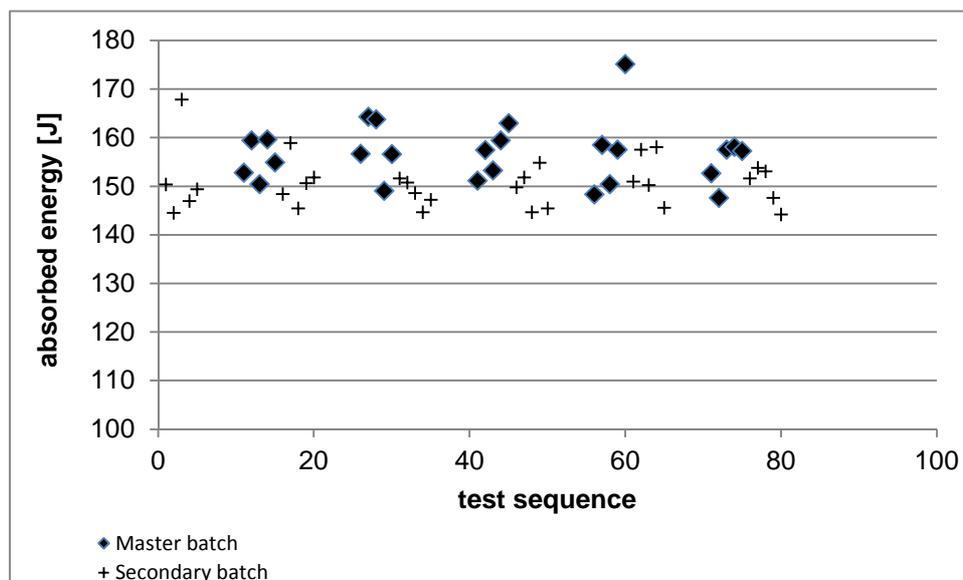
Figure 3: Absorbed energy values of 30 test pieces of ERM<sup>®</sup>-FA415aj, compared with 25 test pieces of ERM<sup>®</sup>-FA415s; data are displayed in the actual test sequence.
