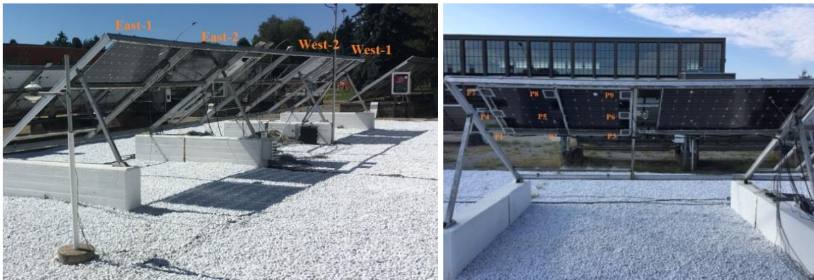
Figure 26: Outdoor set-up for measurement of bifacial PV modules.
