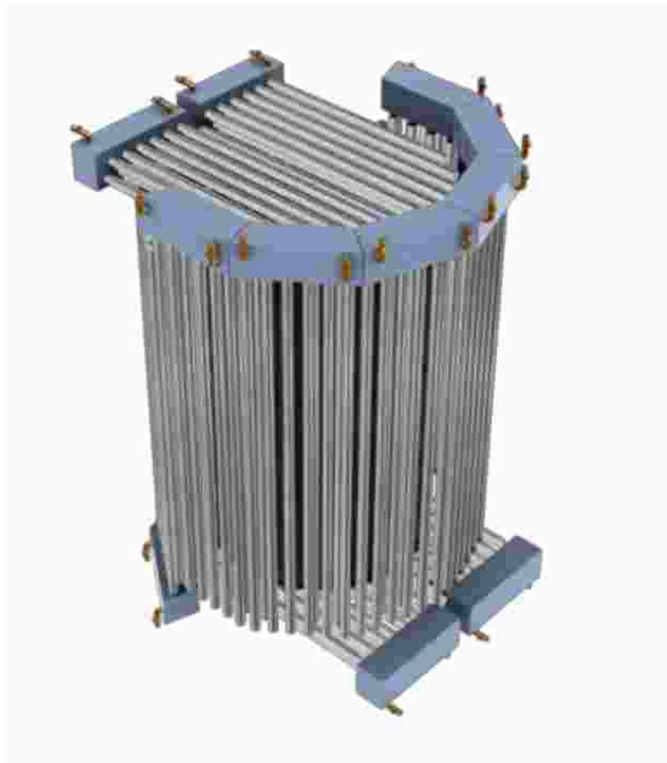
Figure 1. JRC drum monitor ^3\text{He} tube layout
