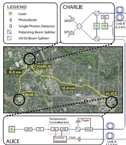
Fig. 31: QKD deployment in Calgary, used to test MDI-QKD. Alice and Bob are connected to Charlie by deployed dark fibres of 12.4 km and 6.2 km length, each of them with a  $\sim 4.5$  dB loss.
