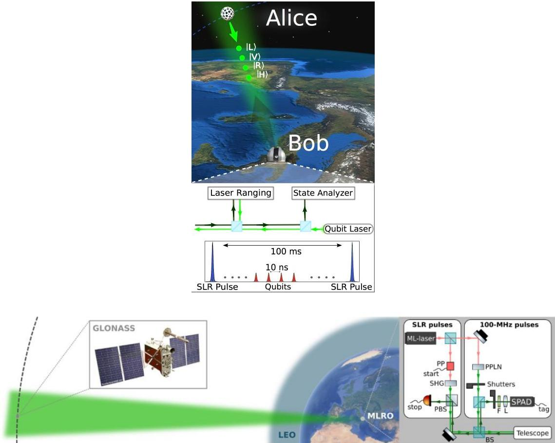
Fig. 16: space quantum communications with LEO satellites and with a GNSS (MEO) satellite.
