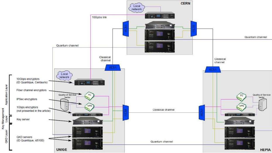
Fig. 13: architectural implementation of the SwissQuantum network.
