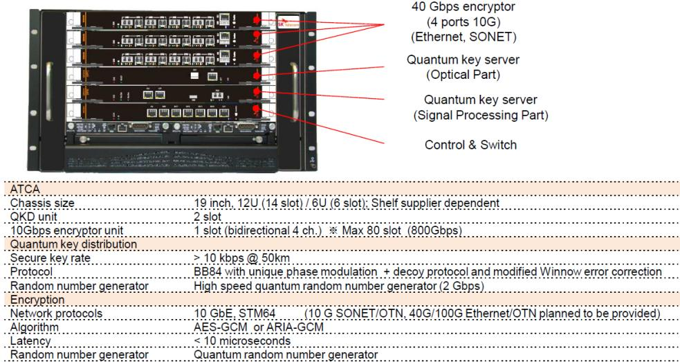
Fig. 7: the QKD system developed by SK Telecom<sup>29</sup>
