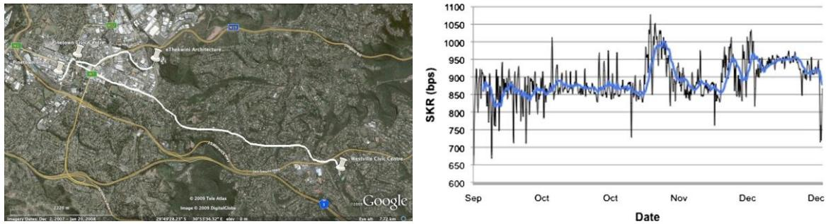
Fig. 33: map of the fibre layout in the QuantumCity project, and secure key rate over the testing period, September to December 2009.
