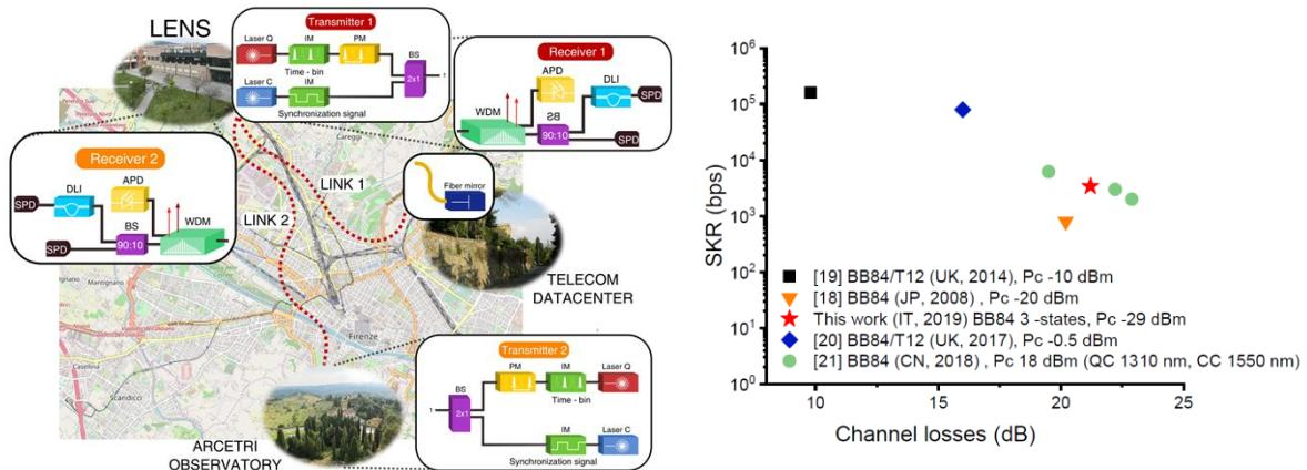
Fig. 15: discrete variable QKD system over 40 km of loop-back dark fibre link (Link 1), and performance comparison with other field experiments<sup>37</sup>. Coexistence with DWDM traffic will be tested on the 21km LINK 2.
