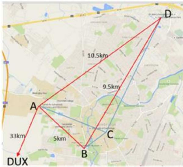
Fig. 21: The Cambridge Fibre network. A: Electrical Engineering building; B: Engineering Department; C: University central network facility; D: Toshiba Research Europe Cambridge Laboratory; DUX: dark fibre link to Duxford.
