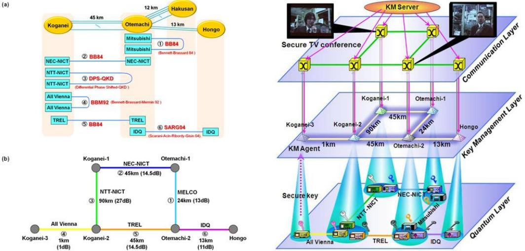
Fig. 5: topology and functional layers of the Tokyo quantum network. A live demonstration of secure TV conferencing, eavesdropping detection, and rerouting of QKD links was performed and made public in October 2010: a live video stream for was encrypted by OTP, with an encryption rate of 128 kbps. Secure keys were provided by over two routes, with total distances of 69 km and 135 km respectively.
