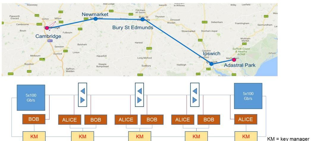
Fig. 20: quantum link deployed between Cambridge and BT labs, with trusted nodes.
