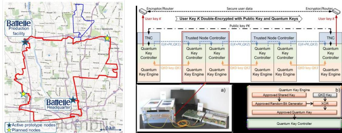
Fig. 26: Batelle QKD network in central Ohio, with a 25 km long loop<sup>64</sup>, and its architectural implementation. The apparatus provides a QKD secret key rate of ~1 kbps over fibre links with less than -19 dB transmission.
