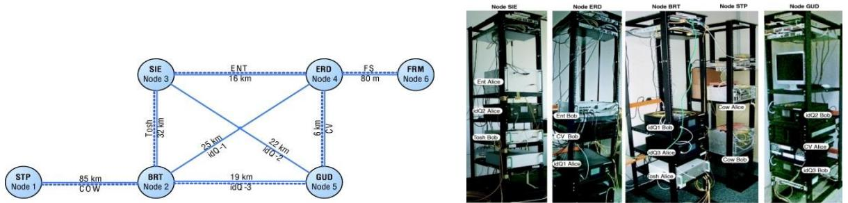
Fig. 9: SECOQC network topology and quantum hardware implementation
