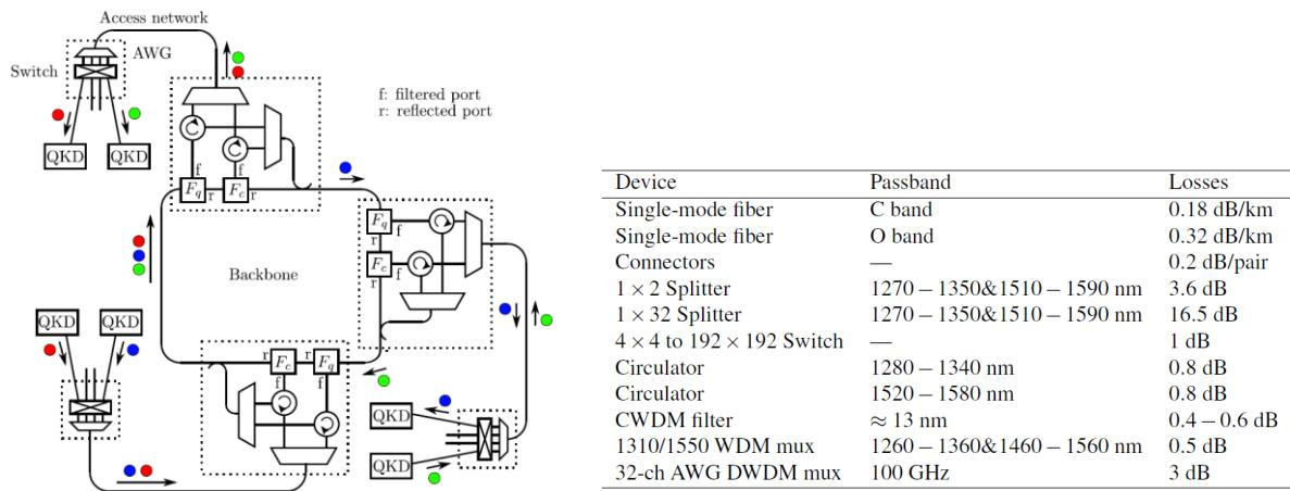
Fig. 17: QKD Metropolitan Area Network with three access networks, and table with the typical optical loss introduced by its components.
