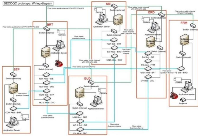
Fig. 11: application layout of the SECOCQ testbed
