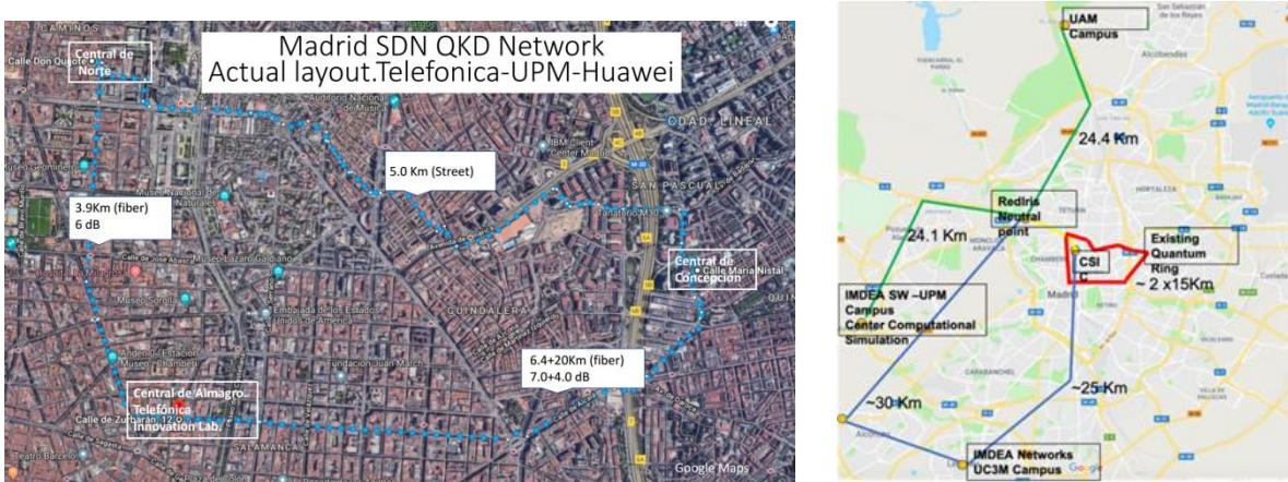
Fig. 18: Core of the Madrid Quantum Network installed in Telefónica Production Facilities, and extended Madrid Quantum Network. The red ring connects the core production facilities, and the yellow link will join the production network with the RedIMadrid network (courtesy Universidad Politécnica de Madrid).
