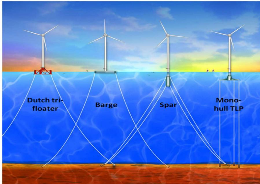
Figure 6 Most common offshore floaters.
