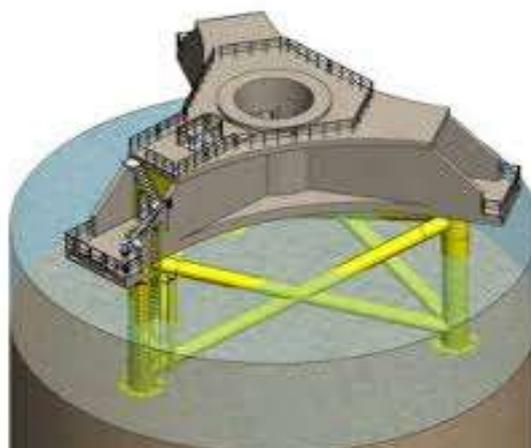
Figure 8 Three-legged jacket foundation with concrete transition piece. Courtesy Siemens
