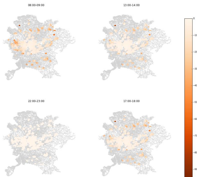
Figure 7: Percentage changes of transport performance due to congestion at different times of the day (starting from top left and moving clockwise: 08:00-09:00, 13:00-14:00, 17:00-18:00 and 22:00-23:00)
