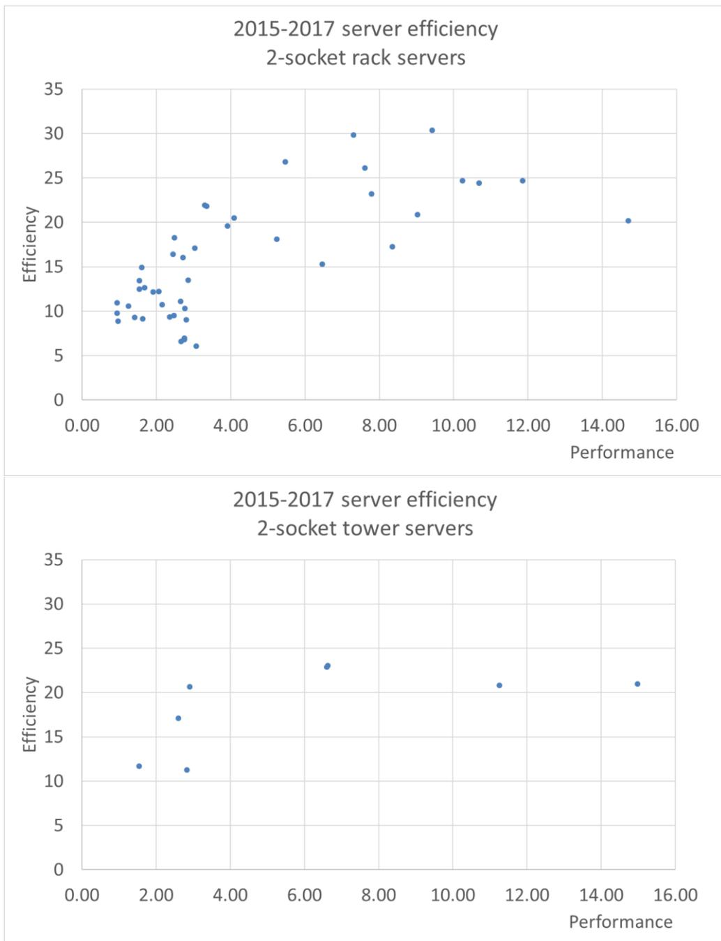
**Figure 13: Analysis of server efficiency by server type carried out in the framework of the Commission Regulation for servers and data storage**
