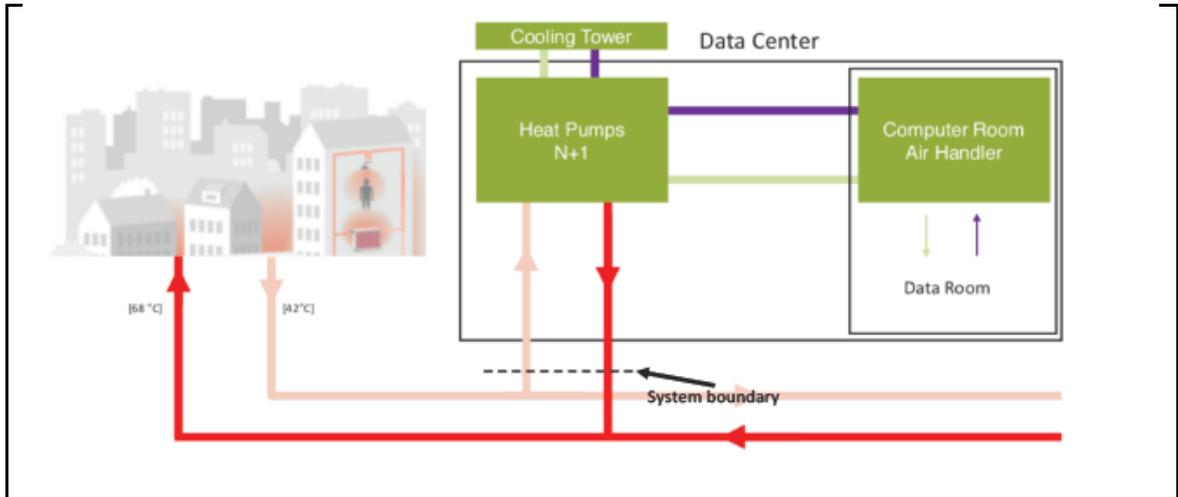
**Figure 18: Example configuration for heat recovery when a data centre is supplying district heating to the city of Stockholm.**
