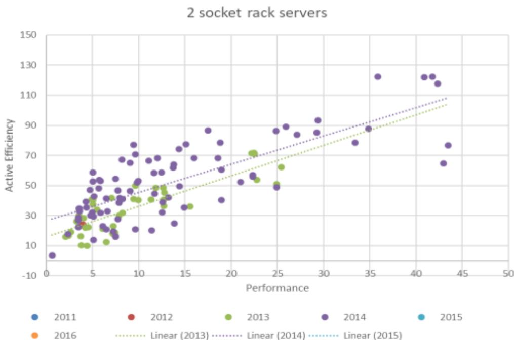
**Figure 12: Relationship between performance (transactions/second) and active efficiency for two-socket servers (transactions/Joule) (higher is more efficient)<sup>38</sup>**
