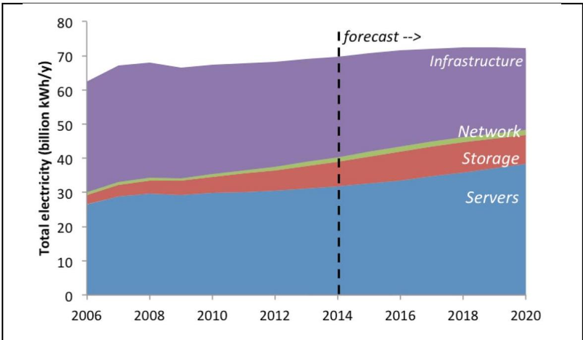
Figure 11: Total electricity consumption by technology type in a data centre<sup>37</sup>
