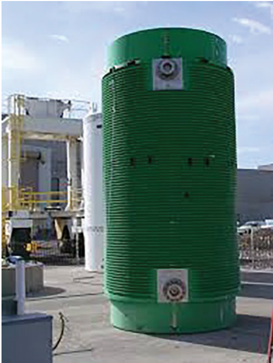
Figure 2: Picture of Castor V/21 which can accommodate PWR 15x15, 16x16 and 17x17.
