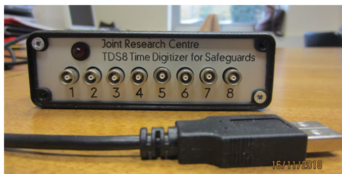
Figure 1: The TDS8 and TDS32 list-mode devices developed at JRC, one with 8 front panel inputs, the other with 32.
