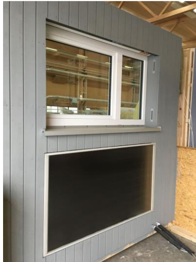
Figure 2. 4RinEu Prefabricated multifunctional façade mockup tested in the lab (credits: Gump&Maier GmbH).
