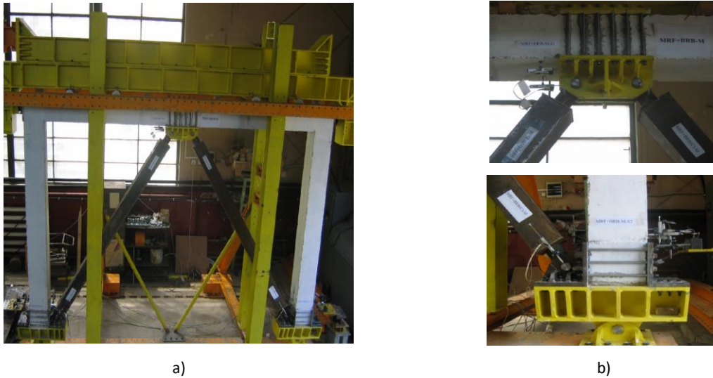
Figure 6. Testing of a full-scale reinforced concrete frame in the PUT laboratory (a) and connection details for installation of BRB in the frame (b).
