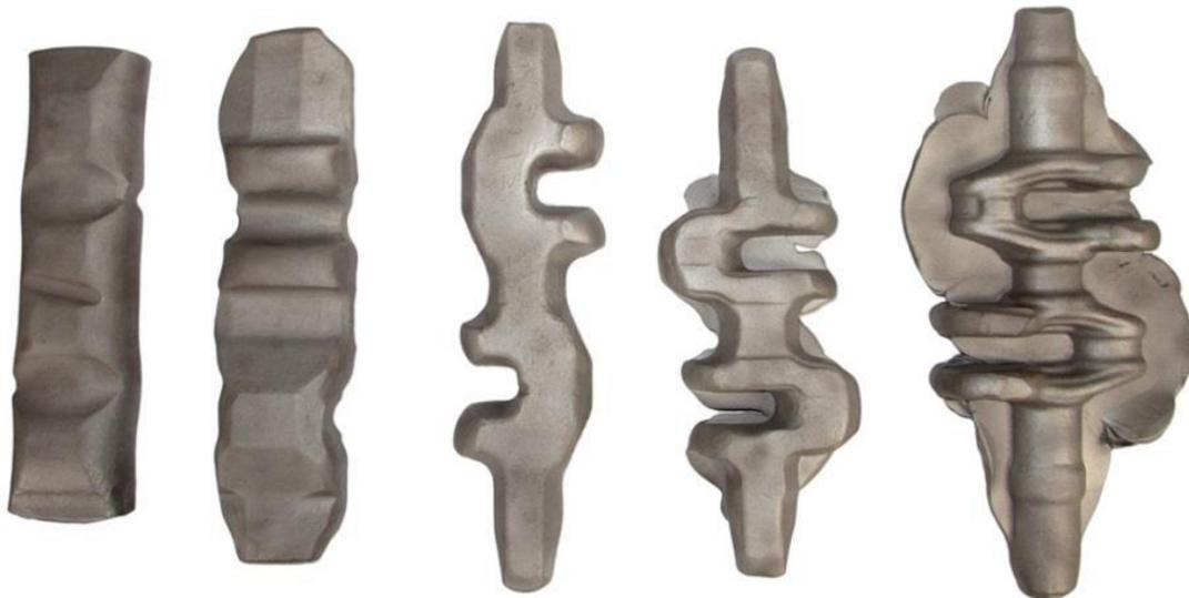
In order to minimise the formation of flash, the complete forging concept, including the forging tools for all the different steps have to be adapted. In the initial forging steps, traditional forging set-up is replaced by “flash free” as shown in Figure 4.26.
