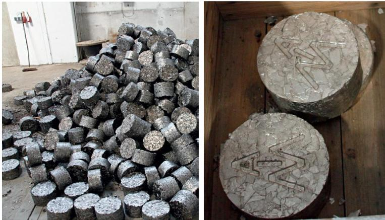
Most briquetting presses are suitable for processing various kinds of swarf resulting from machining of steel, cast iron, stainless steel, aluminium, etc. (keeping in mind the need to avoid contamination if the same machine is used for different streams) and are available in different sizes and filling variants to suit the specific needs of manufacturers and input material. Briquetting can be carried out in-house or outsourced.
