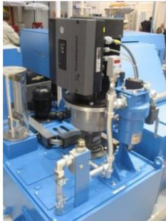
As regards energy efficiency and costs, the flow rate and pressure have to be optimised. In a specific case, the optimum pressure and flow rate were 15 MPa and 31 l/min, respectively. The cleaning efficiency is influenced by the nozzle design, the orifice area and the jet opening angle (Brinksmeier et al., 2015).
