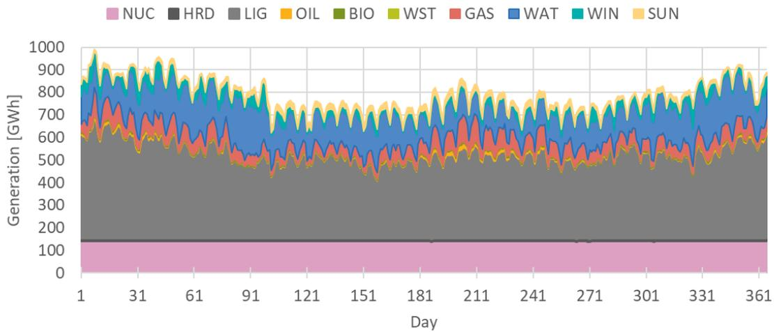
**Figure 11.** Power generation aggregated by fuel for wet (2010) year in GWh
