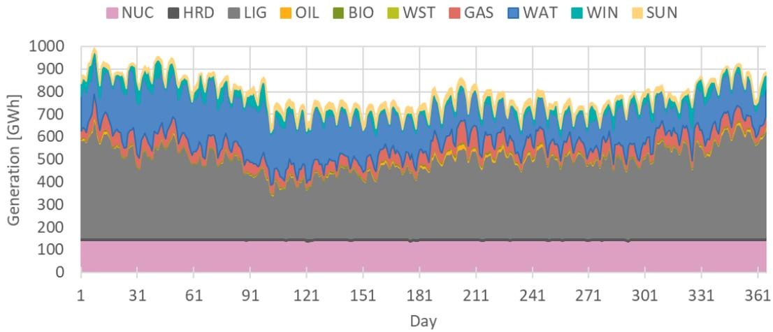
**Figure 10.** Power generation aggregated by fuel for dry (2007) year in GWh
