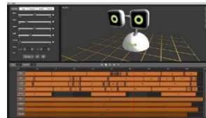
Figure. A routine generator application is used to combine the different actuators of the robot (motion of 5 degrees of freedom) to define the open-loop behaviours.
