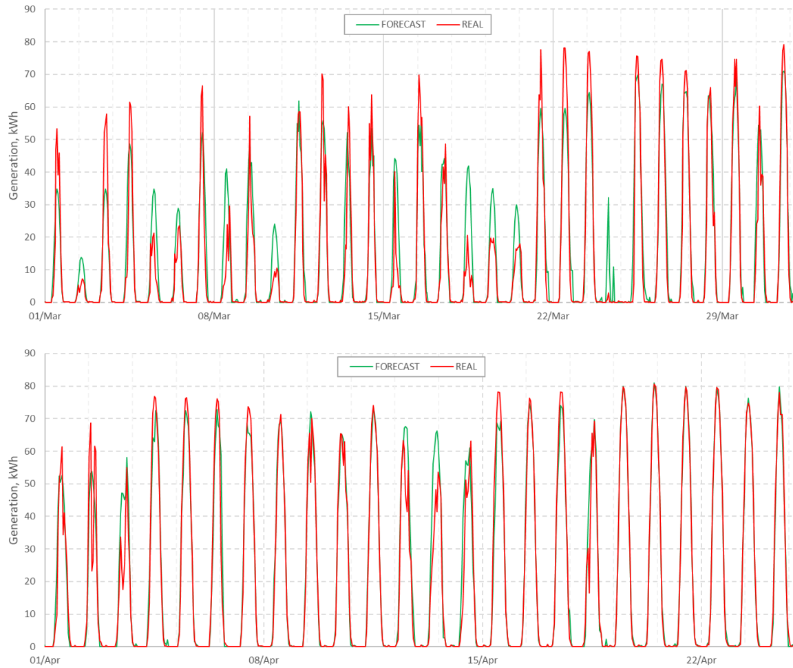
Fig. 11. Forecast prediction graphs for PV generation (March and April 2020)
