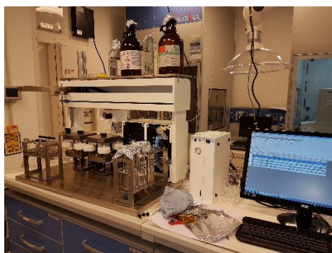
Figure 15. Filter elution on automatic extractor
