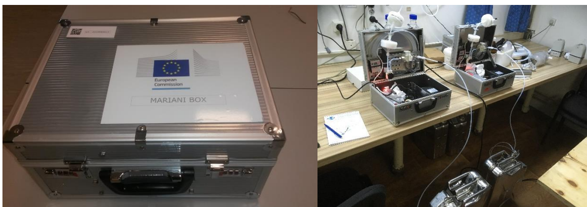
Figure 14. Sampling device used for 20L spot samples
