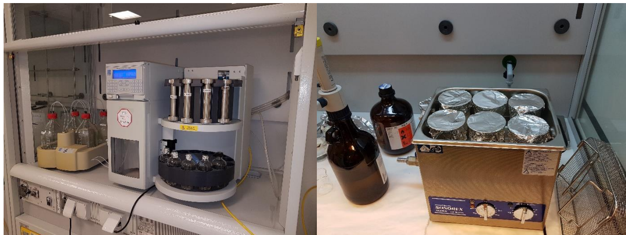
Figure 22. Cells extraction on ASE system and filter extraction on USE system
