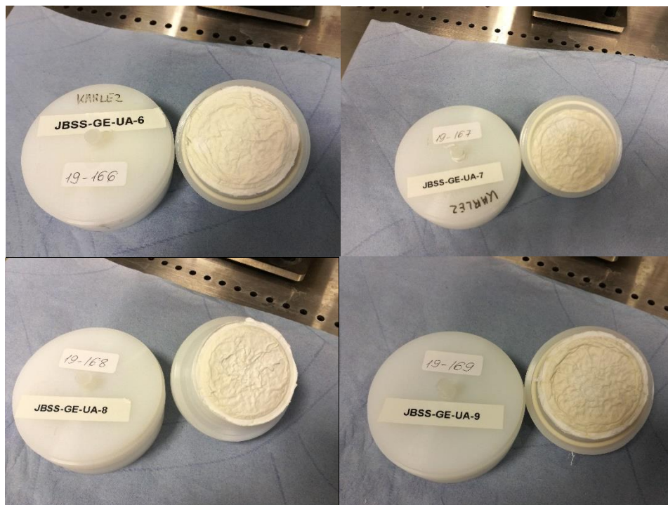
Figure 12. HLB disks used in open sea for samples from JBSS-GE-UA-2 to JBSS-GE-UA-9
