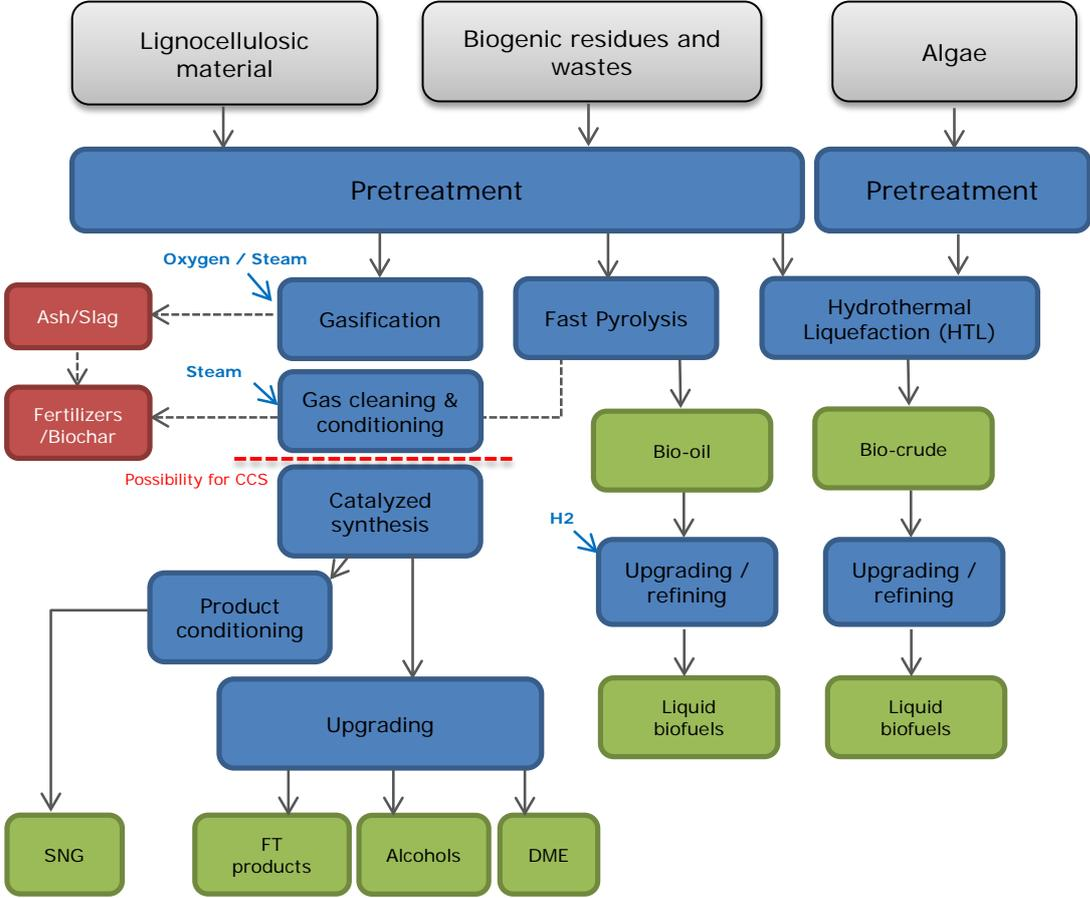
Figure 3. Simplified oleochemical process diagram for liquid fuels production
