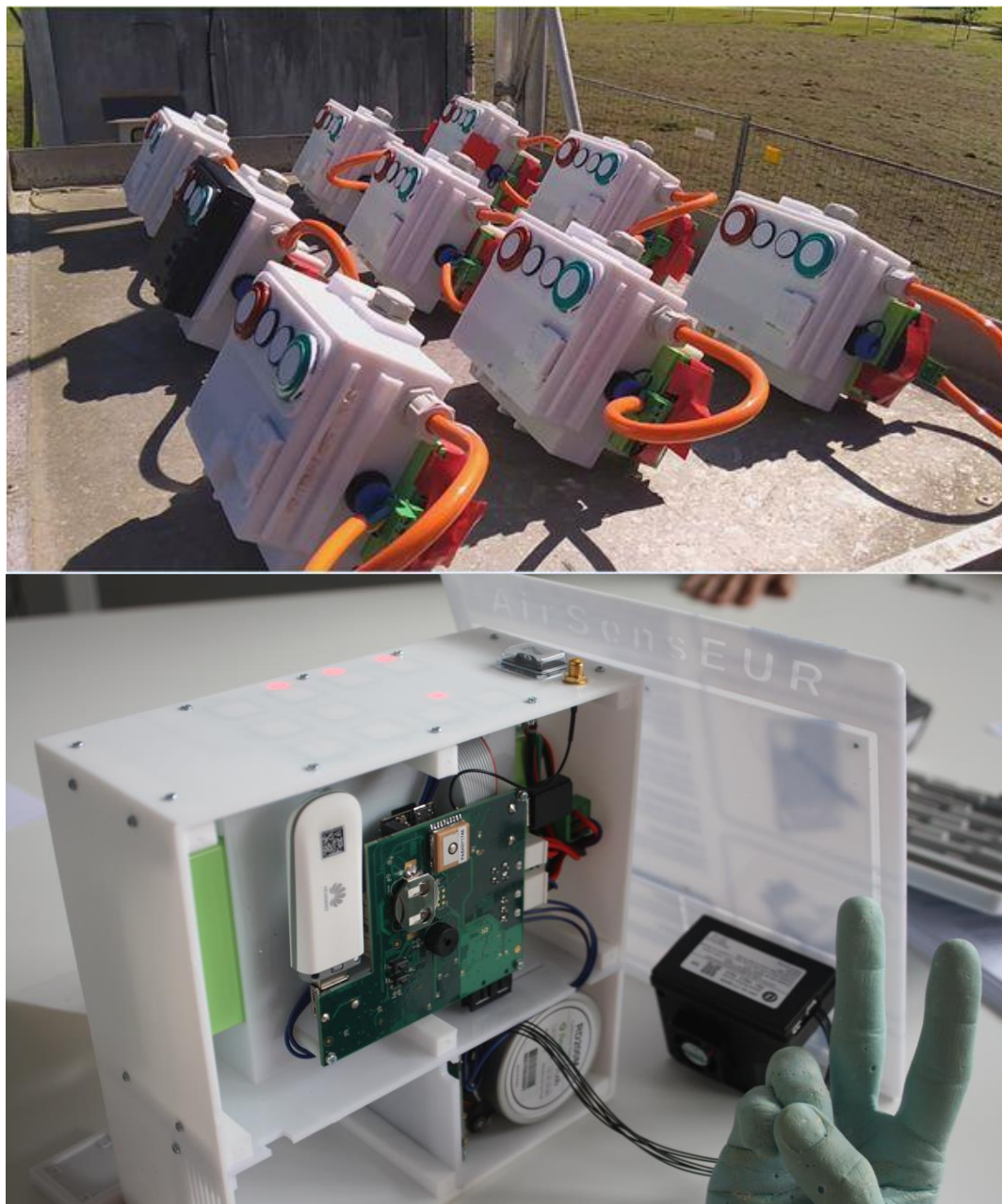
Figure 5. AirSensEUR sensor boxes in action –a deployment of the first version in the Netherlands (on top) and the newest version as presented at the European Clean Air Day 2019 (at the bottom).
