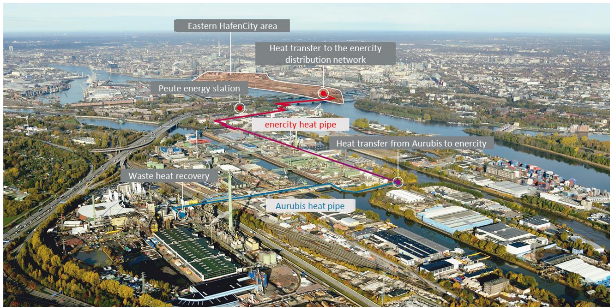
Figure 77: Connection of eastern HafenCity DH with Aurubis waste heat (source: Aurubis)
