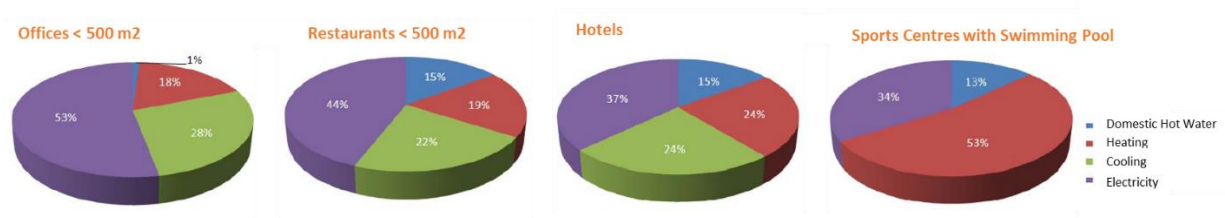
Figure 62: Typical energy consumption of service buildings (source: Districlima Barcelona)
