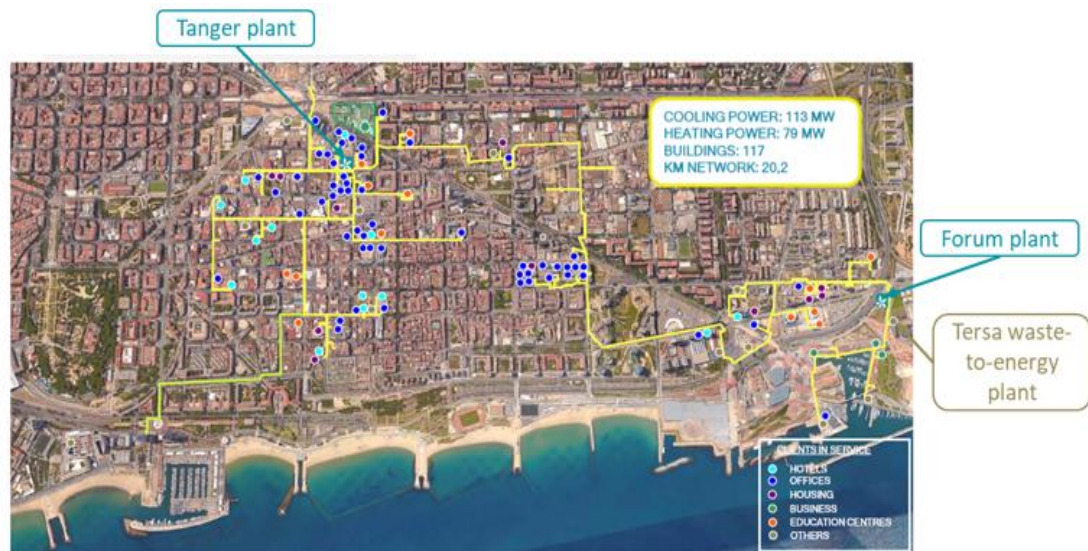
Figure 65: Map of Districlima DHC system, and type of connected buildings (source: Districlima)
