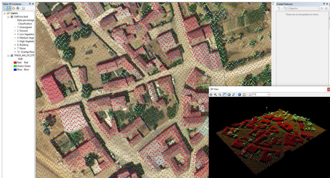
Figure 70. LiDAR cloudpoints with ASPRS code classification
