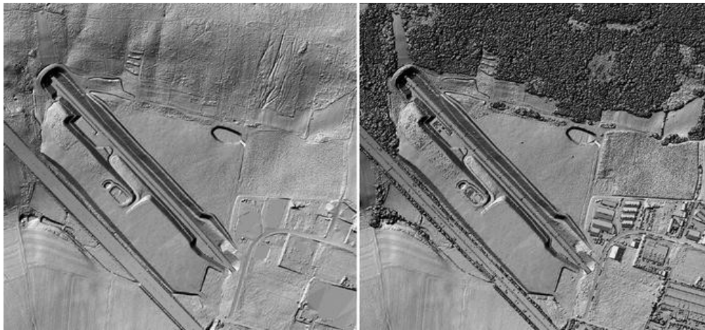
Figure 2. Examples of a DTM (left panel) and a DSM (right panel) (5) .
