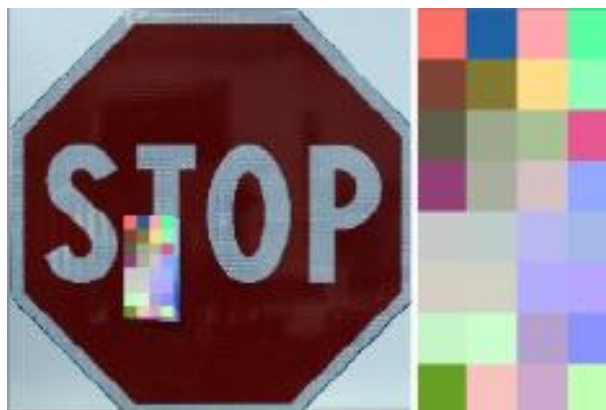
Figure 2 – Adversarial attack against a traffic sign carried out in JRC: a sticker (right) is placed onto a 'Stop' sign (left) causing a traffic sign recognition system to incorrectly classify it as an 'End-of-speed-limit' sign.
