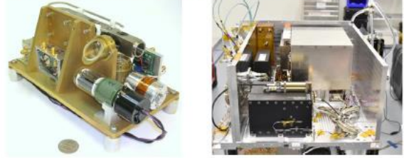
The Deep Space Atomic Clock physical package and the payload (17L, 44W)
