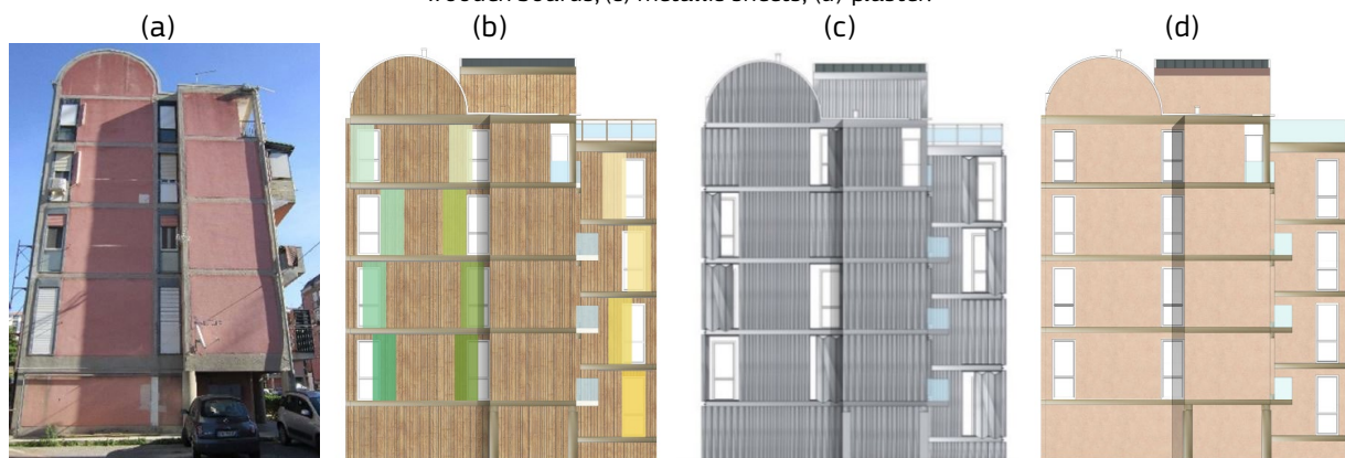
Figure 34. Proposed external cladding for CLT panel retrofit of case study building: (a) current state; (b) cladding with wooden boards; (c) metallic sheets; (d) plaster.
