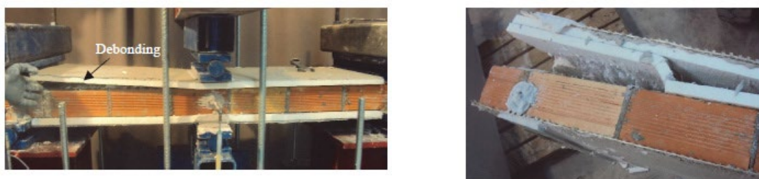
Figure 26. Debonding at the insulation–masonry interface (a) one layer; (b) two layers of insulation.
