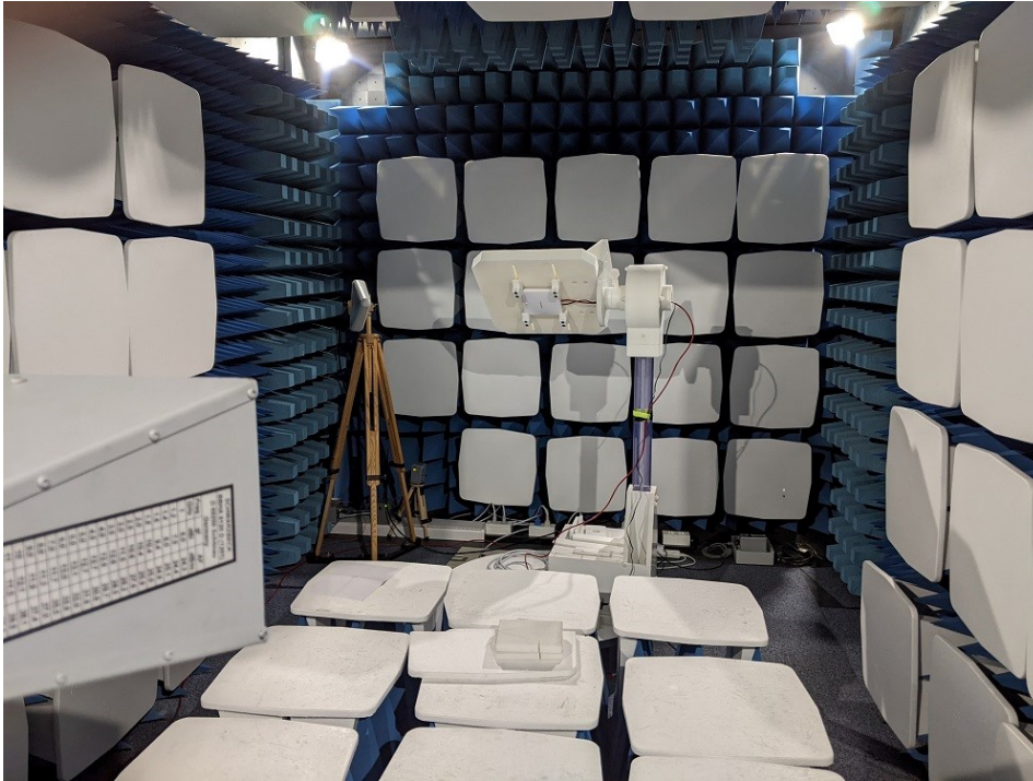
Figure 6: Orientation test in the Shielded Anechoic Chamber.
