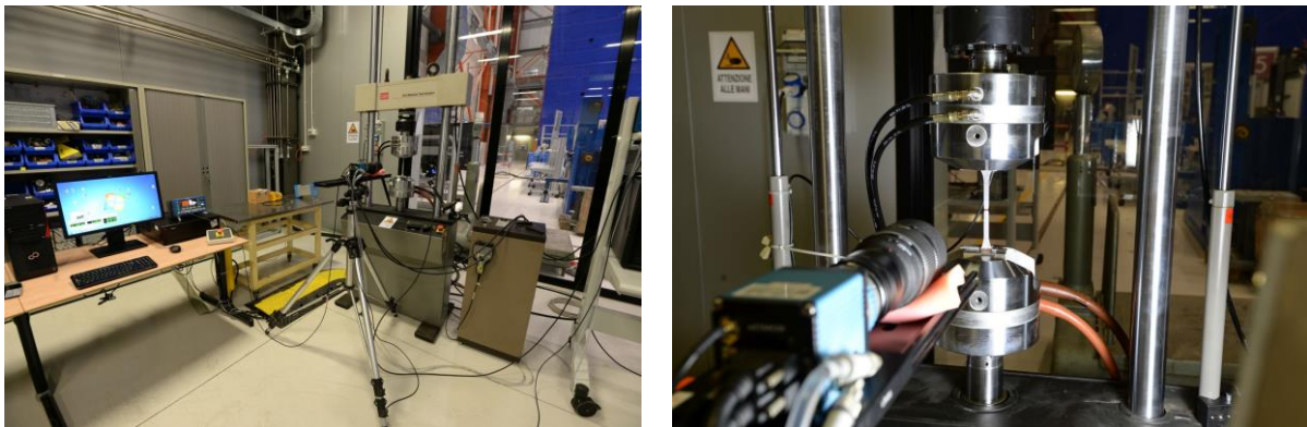
Figure 3. Testing setup for tensile tests on 'standard' geometry specimens (left) and closer view of the specimen and loading equipment (right)
