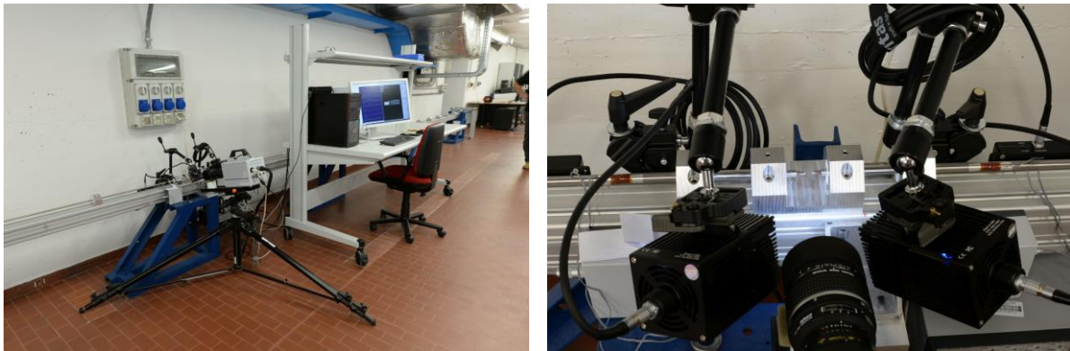
Figure 6. Testing setup for Split Hopkinson Pressure Bar (SHPB) tensile tests (left) and closer view of the specimen and loading equipment (right)
