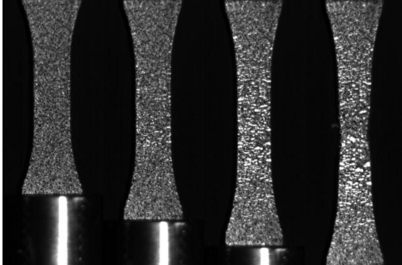
Figure 2. Paint flakes off on copper specimen at 100 mm/s test (b05)
