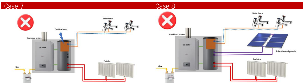
Figure 51. Heating and DHW installations to avoid for in-situ measurements
