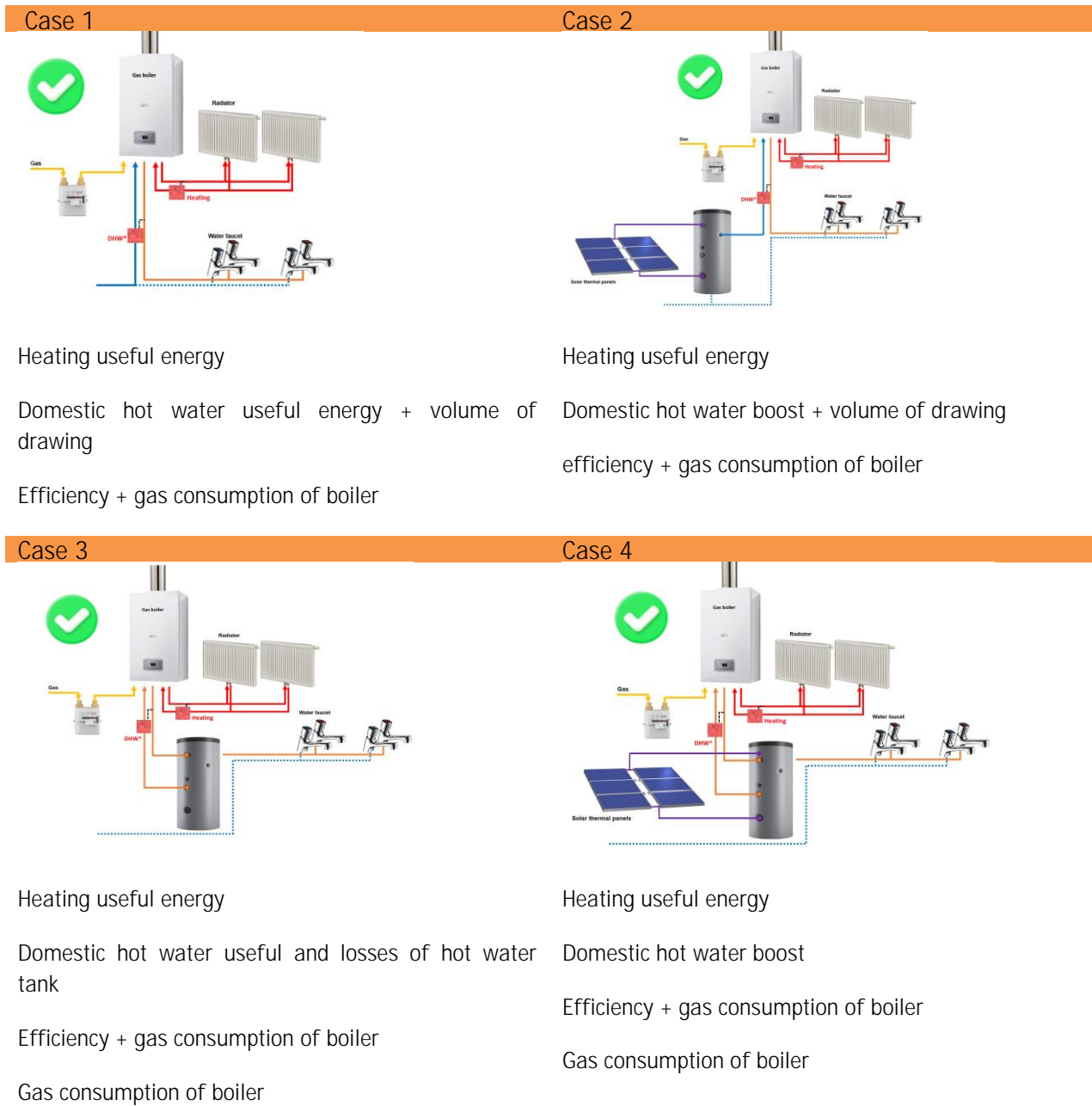
Figure 49. Heating and DHW installations suitable for in-situ measurements
